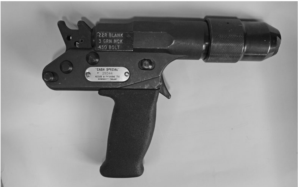
Figure 11.7: The .22 calibre Cash Special is a model of captive bolt widely used on farms and by veterinarians for livestock
