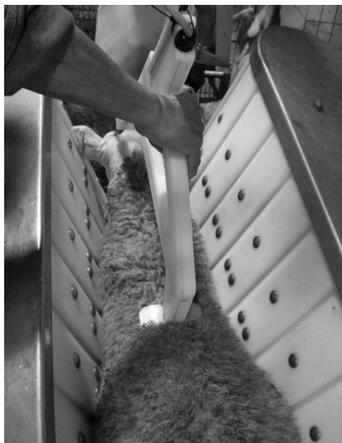
Figure 7.6: Head-to-body electrical stunning applied manually
