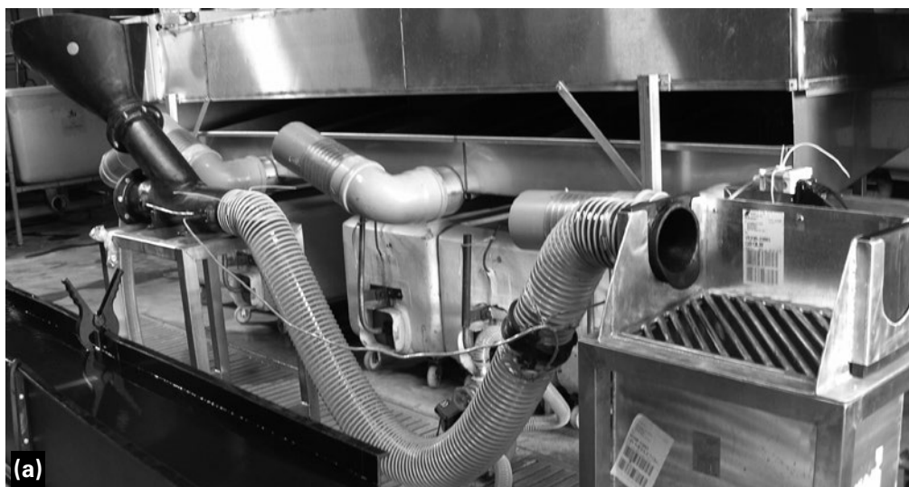
Figure 9.2: Electrical stunning of fish in pipe (a) through which water is pumped to transport the fish through the pipe (b)
