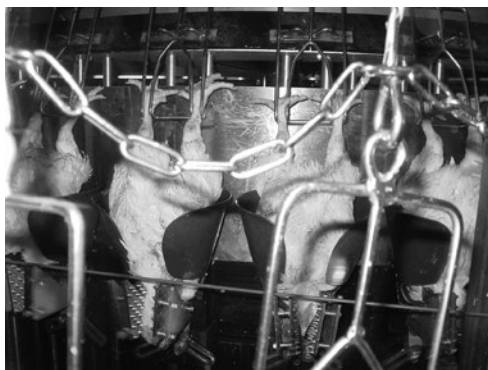
Figure 7.5: Head-only electrical stunning system used for poultry in large-scale slaughterhouses.
