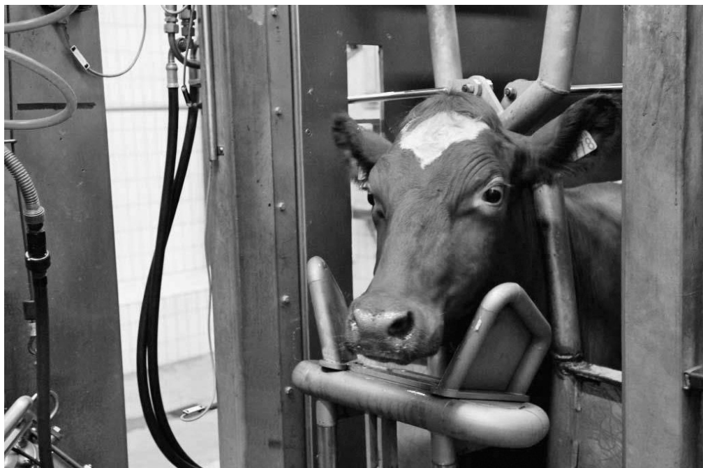
Figure 6.2: Stun box and restraint device with chin lift.
