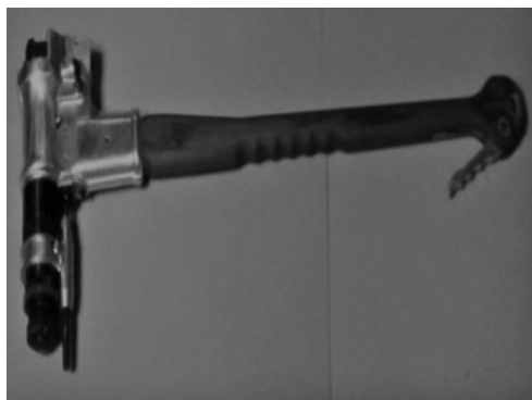
Figure 6.5: Mushroom headed concussion stunner with a trigger
