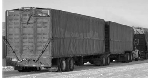
Figure 3.4: Uninsulated tarps on both sides of the trailer are used to protect chickens from the cold, rain or wind.
