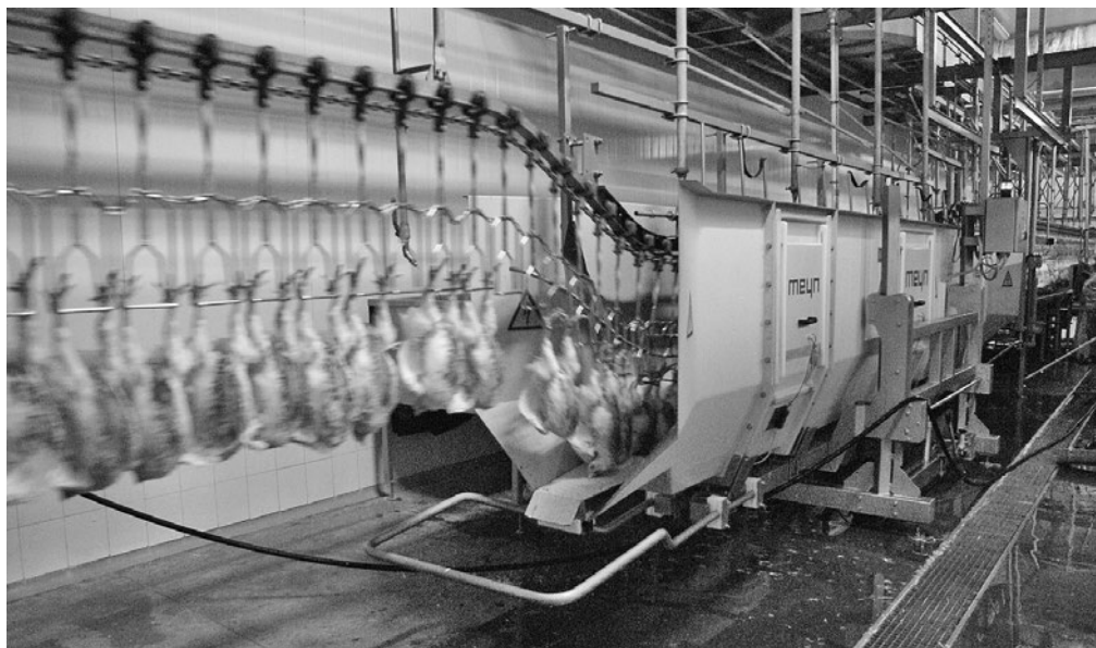
Figure 7.7: Electrical waterbath stunning system used for poultry in large-scale slaughterhouses
