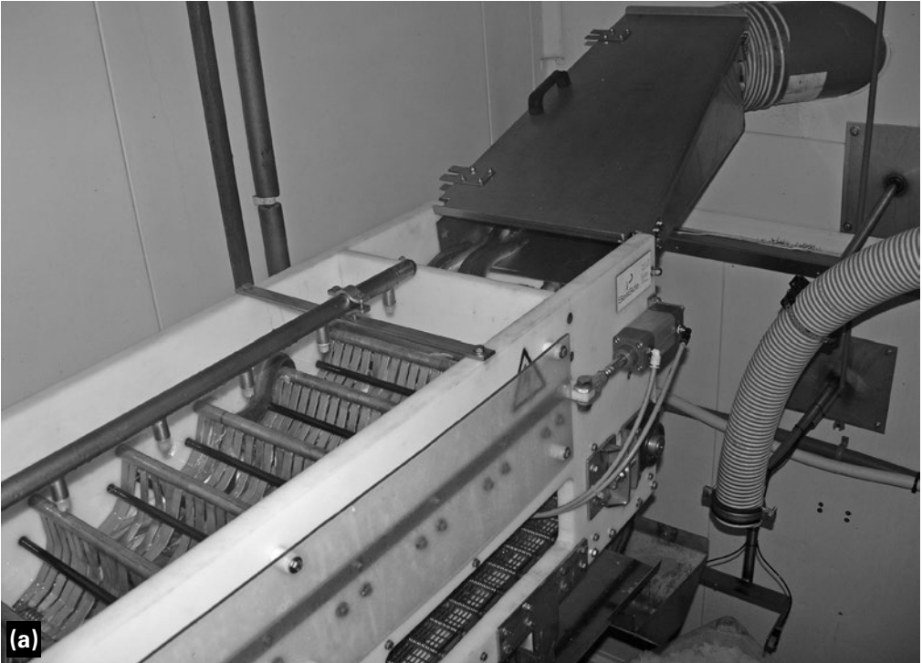
Figure 9.3: (a) Stunner used for electrical stunning of European eel after dewatering; (b) a stunned eel leaving the stunner
