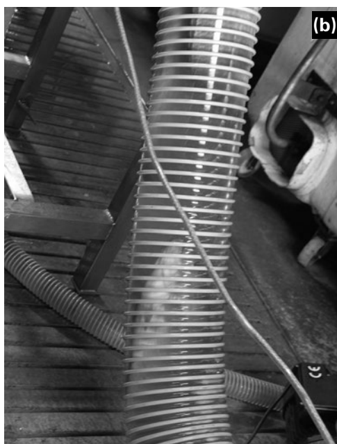
Figure 9.2: Electrical stunning of fish in pipe (a) through which water is pumped to transport the fish through the pipe (b)
