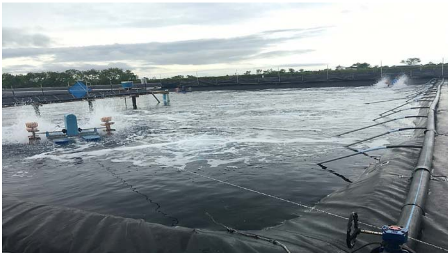
FIGURE 6.7 Additional diffusers from air blowers are often required in a biofloc pond. Credit: K.R. Salin.
