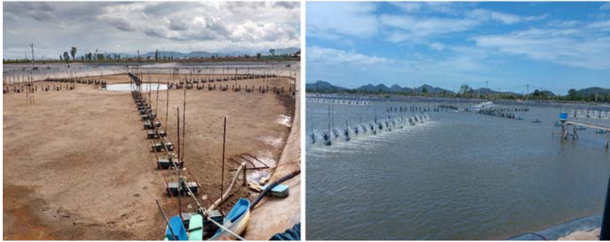
FIGURE 6.6 Proper aeration also helps in sludge removal from the center of a biofloc pond; an empty pond (left) and a fully operational pond (right). Credit: K.R. Salin.
