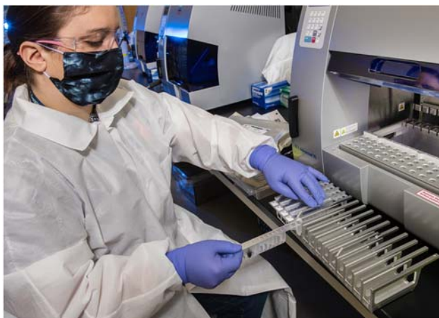
FIGURE 4.2 ID # 24477 CDC/James Gathany, 2020 Public Domain. This Centers for Disease Control and Prevention (CDC) scientist is preparing samples for Real-Time Reverse Transcriptase (RT)–PCR analysis of SARS-CoV-2 specimens. Millions of these test kits have been processed in the United States since the beginning of the COVID-19 pandemic.
