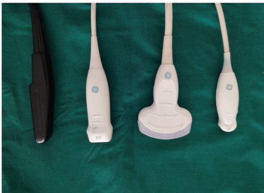
Fig. 7: Showing different types of transducers. From left to right linear transducer 5 MHz with large foot print, linear transducer 3 MHz with small foot print, curvilinear transducer 4 MHz, curvilinear transducer 8MHz
