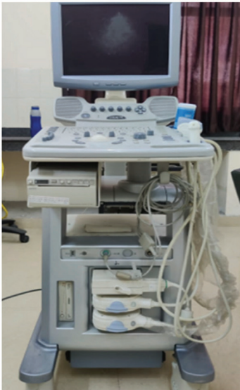
Fig. 140: GE Logic P5 Echocardiographic machine with B-mode, M-mode and Doppler facility.
