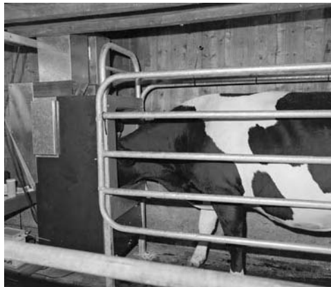
Fig. 25.2. A transponder-controlled feeding stall was modified to allow individual cow breath samples to be taken before feed was dispensed to the cow. Photo: Silsoe Research Institute.
