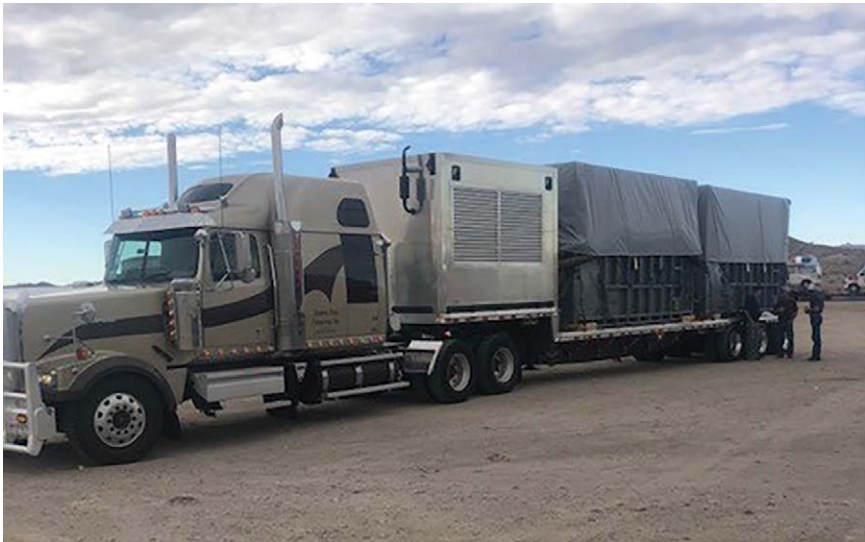
Fig. H2 Heating, Ventilation and Air-Conditioning (HVAC) system installed on a truck large enough to transport two adult elephants. The HVAC is located immediately behind the cab in front of two transportation crates. (Courtesy of Stephen Fritz, Stephen Fritz Enterprises, Arizona).
