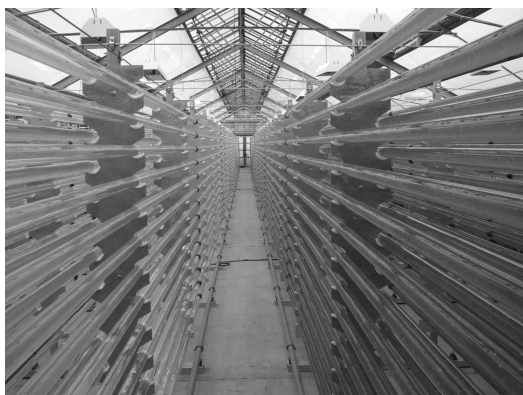
Figure 11.4 Photobioreactor for cultivation of microalgae at IGV GmbH, Germany. (Photo from IGV GmbH, Germany).
