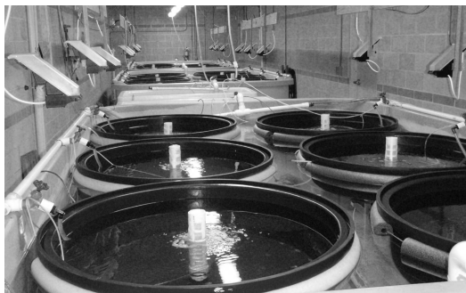
Figure 13.5 Larval fish rearing tanks with automatic feeding system and water movement in the University of Texas Marine Science Institute, Coastal Conservation Association of Texas (UTMSI CCA-Texas) Larviculture Lab in Port Aransas, TX. Six 350-L circular tanks in a 4,000-L rectangular tank (1.2 width \times 2.4 length \times 0.5 height, in meters) with temperature control, biofiltration, sand filtration, aeration, and pumped return water. (Photo by Avier Montalvo, UTMSI.)
