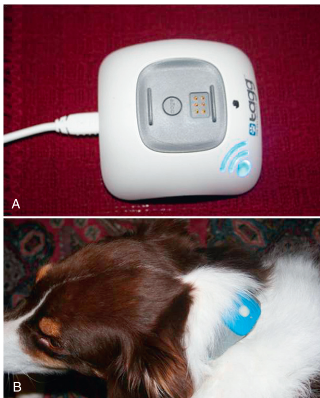
Fig. 3-30 A , Tagg—The Pet Tracker system locator dock, which must remain plugged in near a window for the system to work. B , Tagg tracker GPS unit fitted to the collar of the dog in A . This system excels at providing real-time tracking and movement notification that can be monitored from a smartphone or Tablet device.
