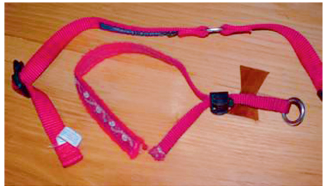
Photo 16 As with all equipment, check your leads, harnesses, collars, and head collars routinely for damage and replace anything that is questionable. Nothing lasts forever, defects occur, and wear is normal. This head collar suddenly tore across a stitched area, but no one was injured. Most companies will replace products that fail like this one did.
