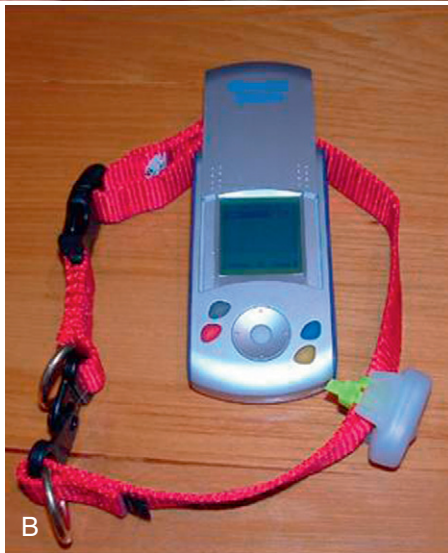
Fig. 3-28 A , An older dog fitted with a transponder for a locator beacon (BrickHouse Security). B , A transponder for the locator beacon is shown attached to a breakaway collar.
