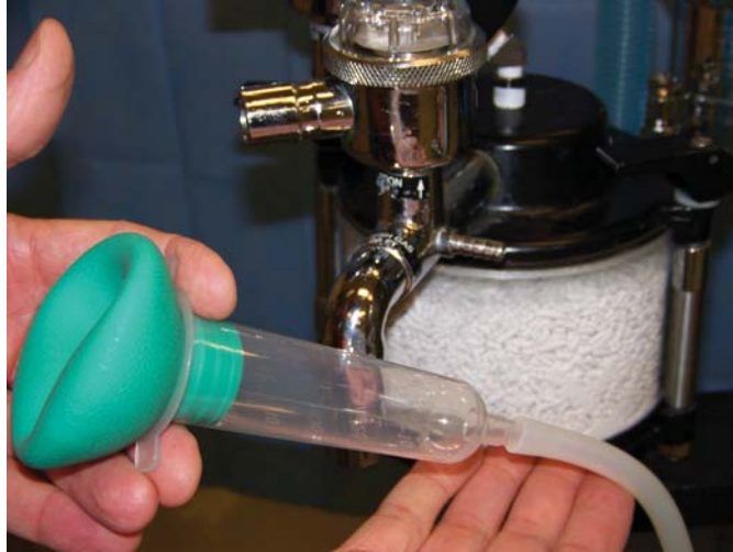
Figure 4.4 Negative pressure leak check: the fresh gas outlet tubing has been disconnected from its attachment to the circle system. A surgical suction bulb is compressed, inserted into the tube, and released. The bulb should remain depressed for at least 10 s indicating a negligible leak (see text for further explanation).
