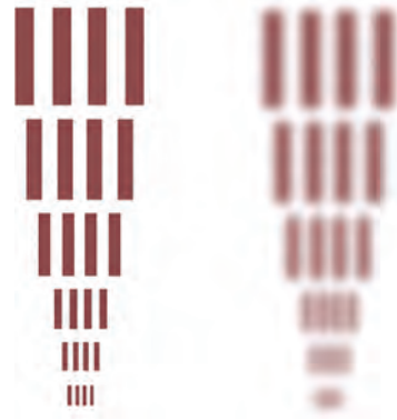
■ FIGURE 4-19 Line pair phantoms are used for practical estimates of the spatial resolution in field tests of clinical imaging equipment. An ideal test phantom ( left ) is imaged, and the system blurs the image of the object as shown here ( right ). The observer reads the spatial frequency (not indicated here) corresponding to the smallest set of bars that were visible, and this measurement is considered the limiting spatial resolution .
