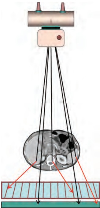
■ FIGURE 7-22 The antiscatter grid is located between the patient, who is the principal source of scatter, and the detector. Grids are geometric devices, and the interspace regions in the grid are aligned with the x-ray focal spot, which is the location where all primary x-ray photons originate from. Scattered photons are more obliquely oriented, and as a result have a higher probability of striking the attenuating septa in the grid. Hence, the grid allows most of the primary radiation to reach the detector, but prevents most of the scattered radiation from reaching it.
