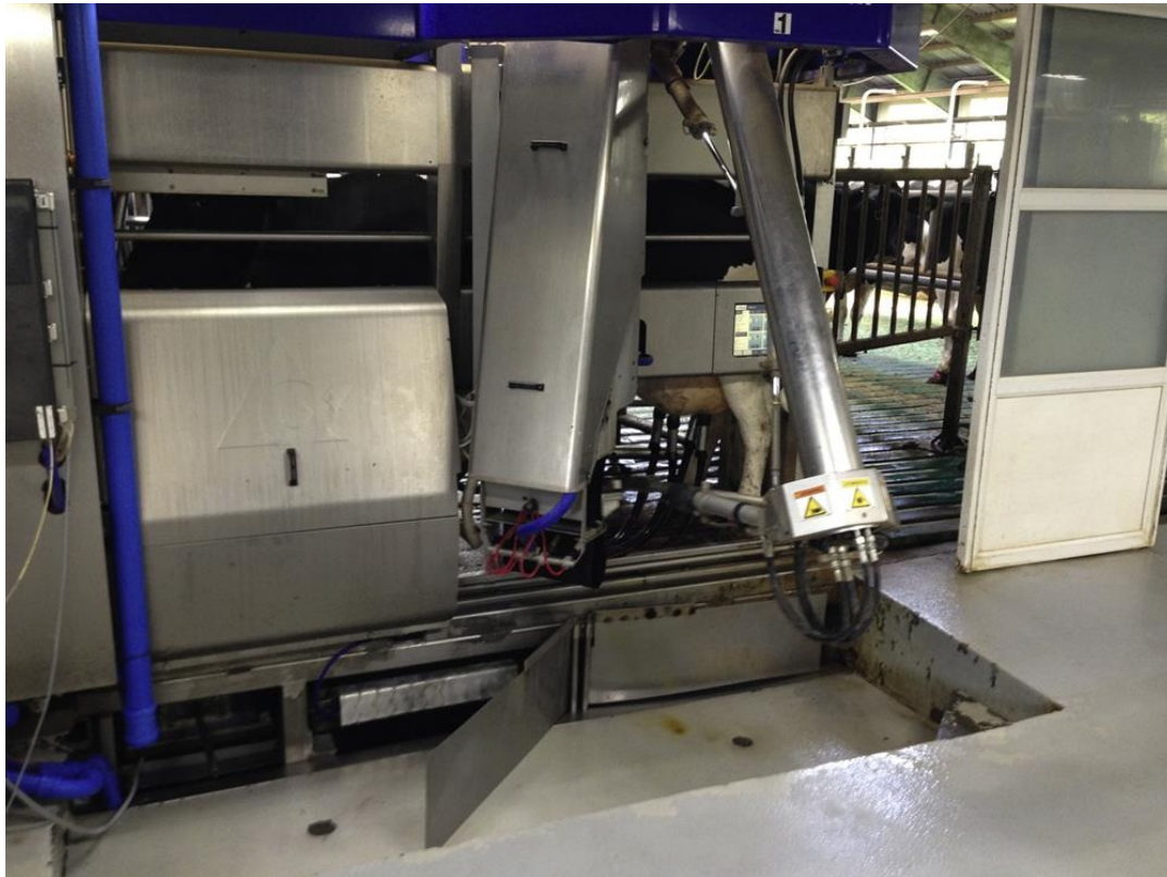
FIGURE 1.7 Cow being milked voluntarily in a robotic milking system box. Source: Photo courtesy of Dr Marcia Endres, University of Minnesota, USA.
