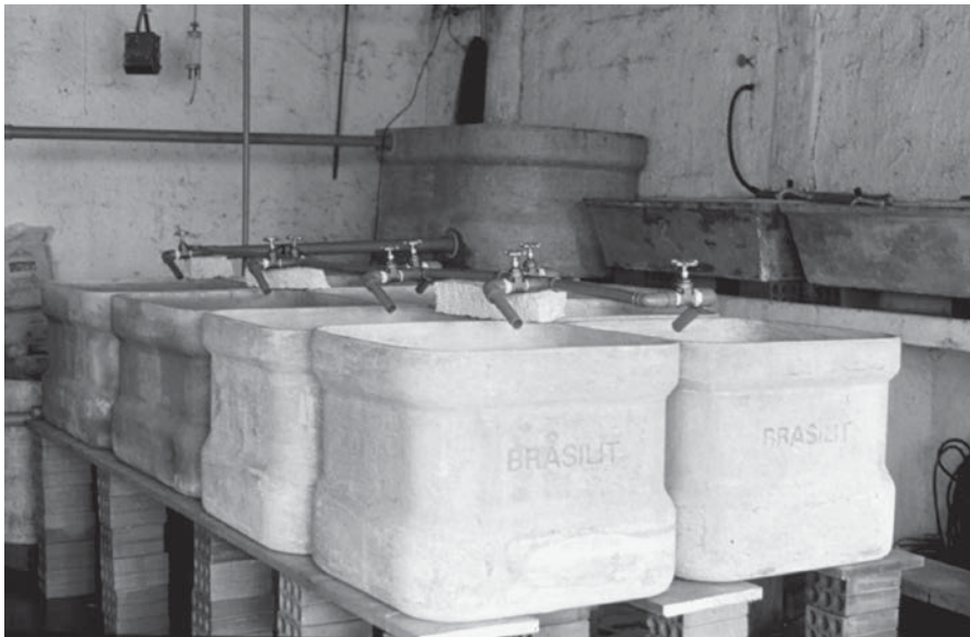
Fig. 3.25. Cisterns make convenient culture tanks in this university research laboratory in Brazil. The tank that is higher than the others is a head tank to provide water to the tanks under some pressure. Other components employing cisterns were the biofilter and settling tanks. Everything was off-the-shelf at the plumbing store.
