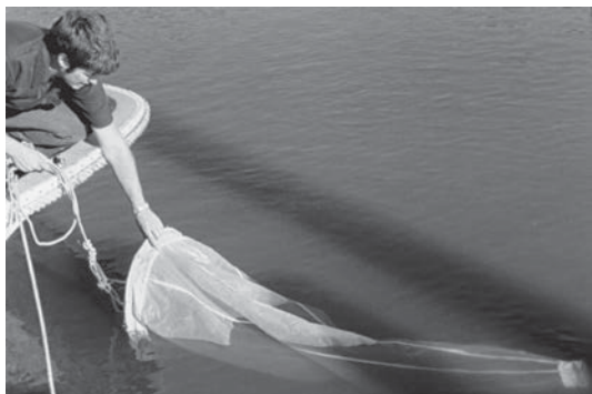
Fig. 6.40. Plankton nets can be used to collect wild zooplankton. The nets are available in various mouth diameters (with 0.5 and 1.0 m being common) and mesh sizes. A cup at the end of the net collects the sample.
