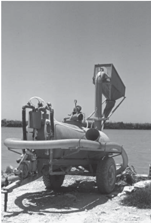
Fig. 9.11. An example of a fish pump. There are many designs and sizes used around the world. This one happens to have been in Israel.
