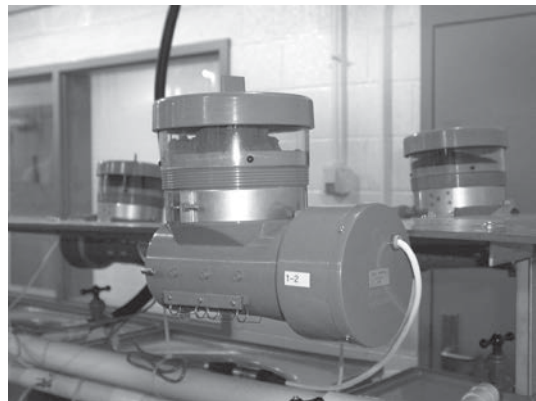
Fig. 7.15. A commercially available automatic feeder. Such feeders operate periodically and are timer controlled.
