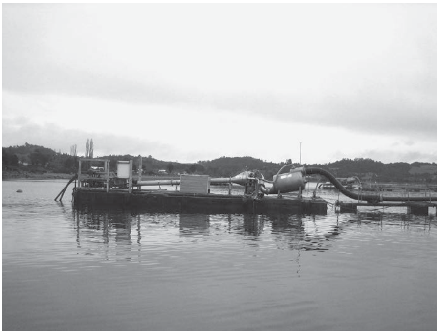
Fig. 9.15. A fish pump at an Atlantic salmon net pen facility in Chile pumps harvested fish from a 'resting' pen into a chilling tank outside the processing plant.
