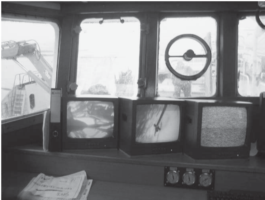
Fig. 7.21. Television monitors on the bridge of the feed distribution boat allow the culturists to observe pictures from multiple cameras simultaneously. Location was a salmon farm in Chile.
