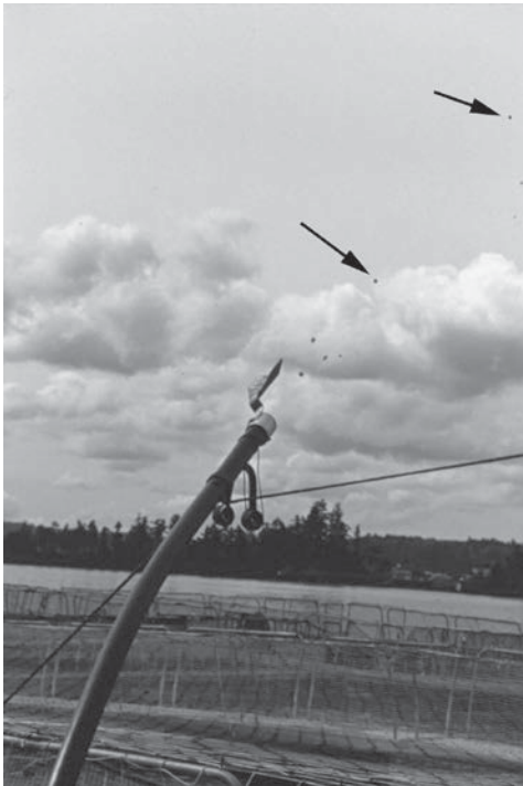
Fig. 7.19. The end of a feed distribution line at a salmon farm in the state of Washington, USA. A few feed pellets that have been blown from the pipe can be seen (two of them are pointed to by arrows). In this case the blower and bulk feed are located on land adjacent to the culture site.
