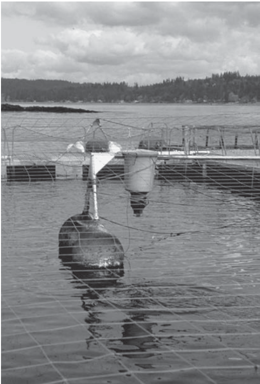
Fig. 7.13. A demand feeder held in position by floats in an Atlantic salmon net pen.
