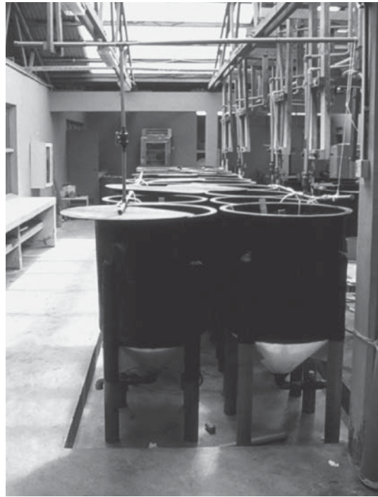
Fig. 6.25. A row of conical bottom shrimp-hatching and larval-development tanks in a commercial hatchery.
