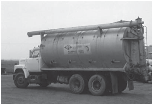
Fig. 7.9. A bulk feed delivery truck used to haul catfish pellets from the feed mill to storage bins on fish farms.
