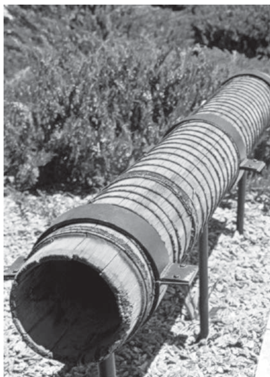
Fig. 3.9. A section of wooden pipe on display at a fish culture facility in Idaho, USA. This type of pipe was used in some of the hatcheries dating back to the 19th century.
