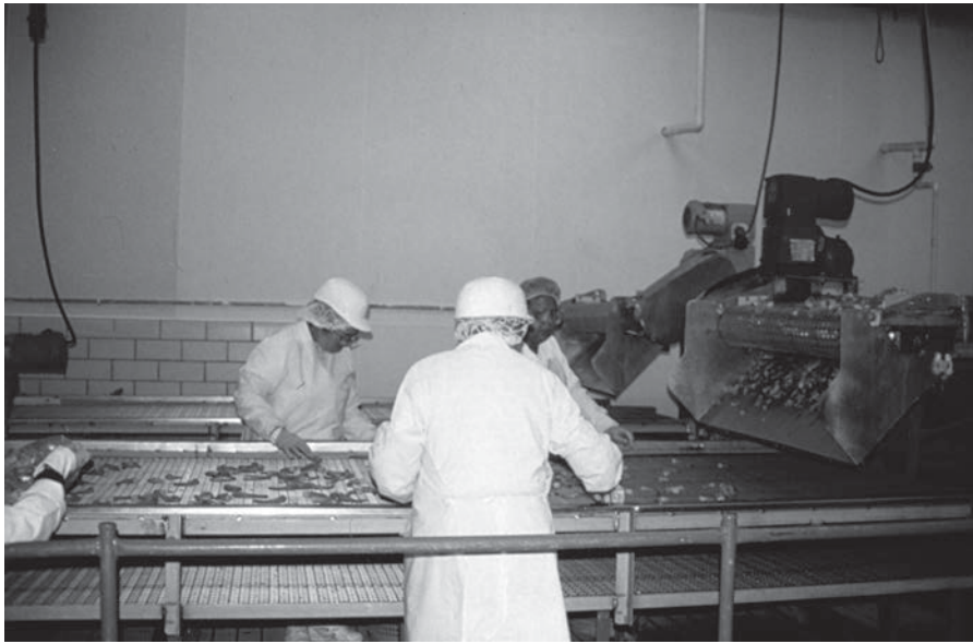
Fig. 9.29. Workers sorting shrimp into size groups in a processing plant.
