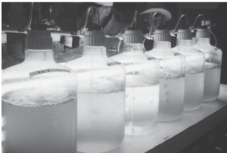
Fig. 3.24. Carboys being used to culture algal cells. The carboy at the left is conspicuously darker, indicating that the cell density is significantly higher than in the other carboys shown. If the photo were in colour, various shades of green would be apparent.
