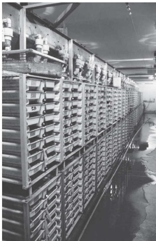
Fig. 4.13. A battery of Heath trays. Each tray can hold several thousand trout or salmon eggs. Water enters each stack of trays at the top and cascades down through the stack.
