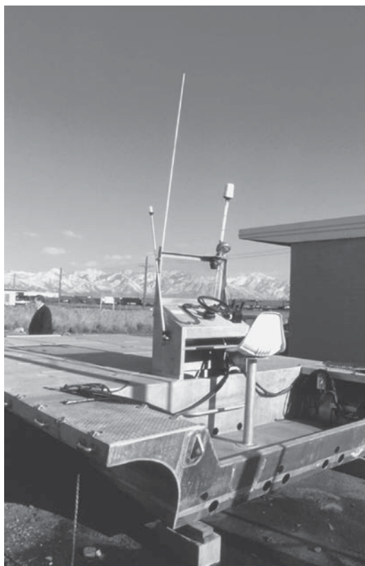
Fig. 6.43. One of the various types of boats used to collect brine shrimp cysts on the Great Salt Lake in Utah, USA. Large tanks are placed on the barge-like boat and the cysts are pumped into them.
