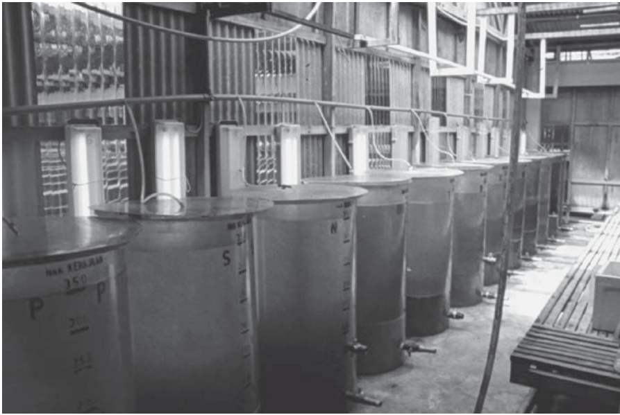
Fig. 6.26. Algae culture tanks with the blooms at various stages of development in a commercial shrimp hatchery. Note the fluorescent light fixtures associated with each transparent tank to promote photosynthesis. The algae are added to larval-rearing and nursery tanks in conjunction with the green water technique.
