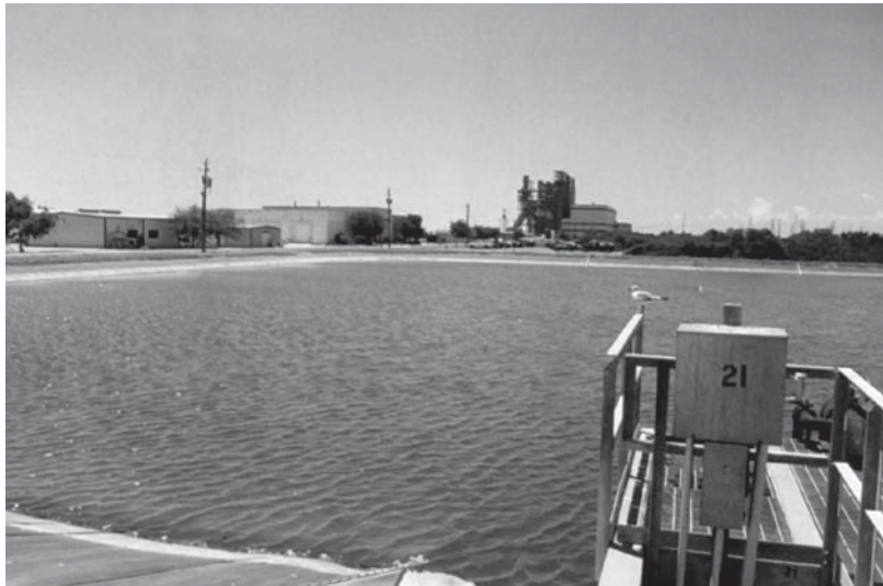
Fig. 6.21. A red drum fry-rearing pond. The one shown is fitted with a plastic liner to prevent seepage through the sandy coastal soil.
