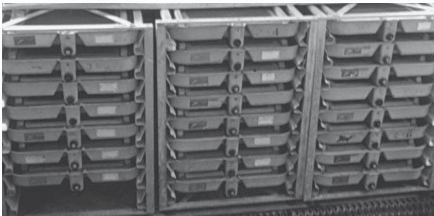
Fig. 6.6. A battery of Heath trays, a type of hatching tray system often used in salmon and trout hatcheries.
