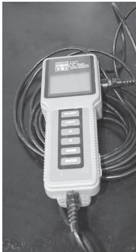
Fig. 4.1. A dissolved oxygen meter (showing the controls and readout area) lies atop the cable that sends data to the meter from a probe at the far end, which is lowered into the water.
