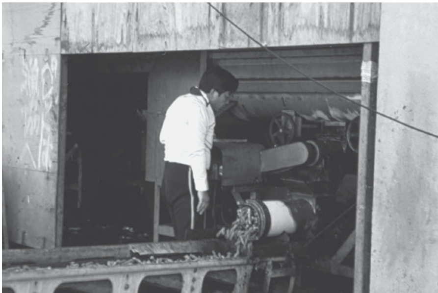
Fig. 7.2. Small trash fish at this fish farming cooperative in Japan are ground up, mixed with about 10% dry ingredients and made into moist pellets by running the mixture through a meat grinder.
