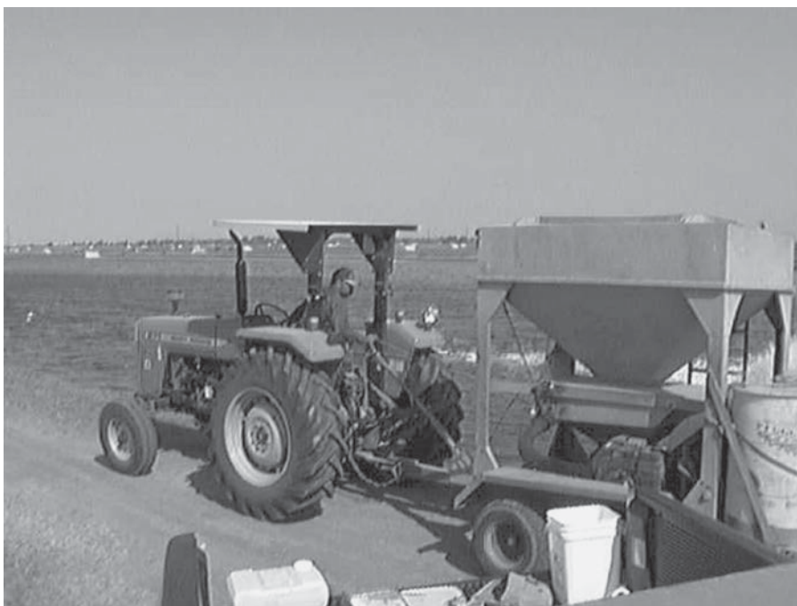
Fig. 7.12. A tractor pulling a mechanical feed blower on a pond bank. The blower is often operated from the power take-off of the tractor in such situations.
