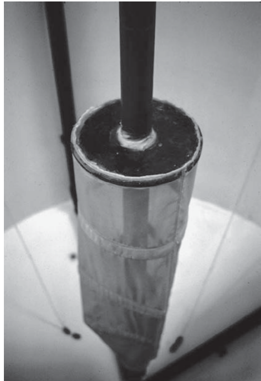
Fig. 3.23. In this tank, the typical outside standpipe has been replaced with one almost entirely comprising fine mesh nylon screen, providing a large area for exiting water to flow through. This reduces the possibility of sucking eggs or larvae against the mesh.
