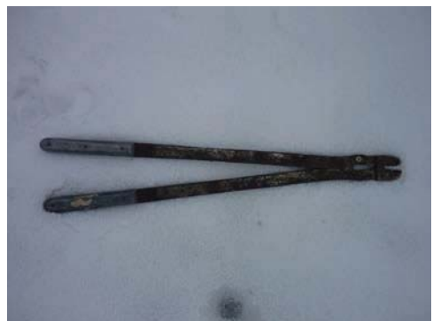
Fig. 4.6. Large horse molar cutters for cutting tusks.
