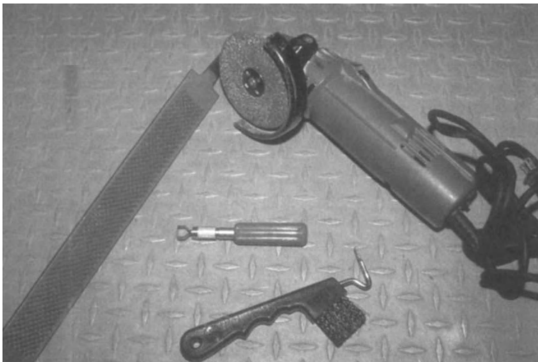
FIG. 7.4—Tools used in foot trimming. Clockwise from left to right: rasp, electric grinder with sanding disc, hoof pick and brush, carving handle with X-acto blade.
