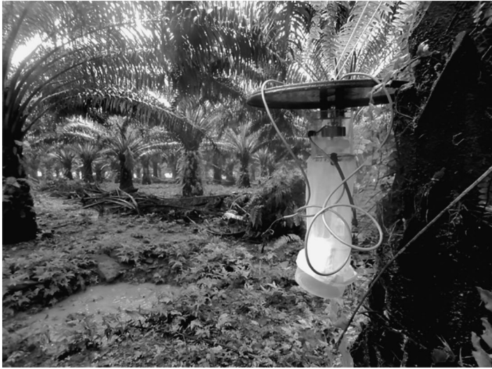
Figure 2. Picture of a CDC light trap installed in a palm oil plantation to collect vectors and identify their associated diseases in highly disturbed habitat after deforestation. © Rafael Gutiérrez-López.
