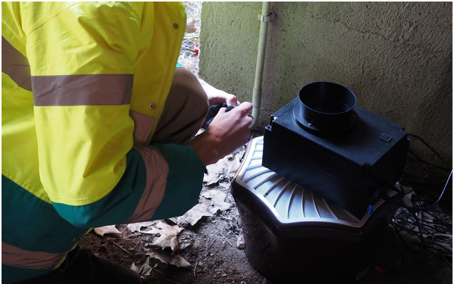
Figure 3. Vector control technician installing a trap with IRIDEON's smart mosquito sensor.
