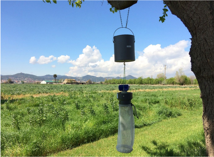
Figure 1. Classic EVS mosquito trap baited with a container with CO 2 pellets.
