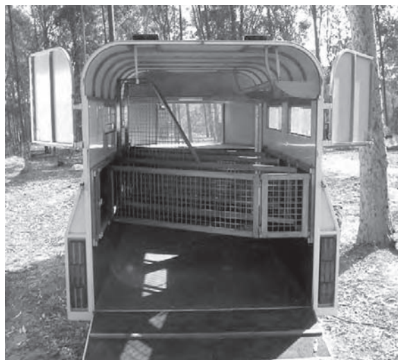
Figure 5. Inside a triple angle load float with barn doors, large tail lights and a rug rack
