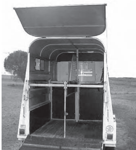
Figure 3. Inside a double float, showing a shoulder partition, rump bars and a door above that operates with gas struts (courtesy of Jane Myers).
