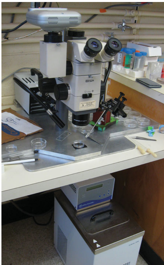
Fig. 2.9. Live-embryo workstation. Stereomicroscope with digital camera mounted from side port. Microscope rests on a custom-built aluminum cooling stage which was channeled to circulate coolant from the temperature-controlled water bath located below the table. Note arrangement of fiber lights, micromanipulator, and embryo dishes on stage.
