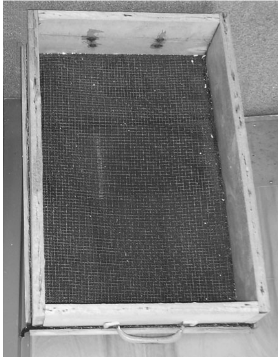
Fig. 16.2. Sieve made of 1'' \times 4'' boards for collecting amphioxus in fine sand. The dimensions of the sieve are 12'' wide by 18'' long. Nylon window screening [standard mesh with 18 \times 16 openings/in. (2.54 cm)] is fastened over the wooden frame with a staple gun. Wire mesh with 1/4–1/3'' meshes is nailed over the window screen. Thin moldings are nailed over the edges of the screen to hold it in place and hide sharp edges.
