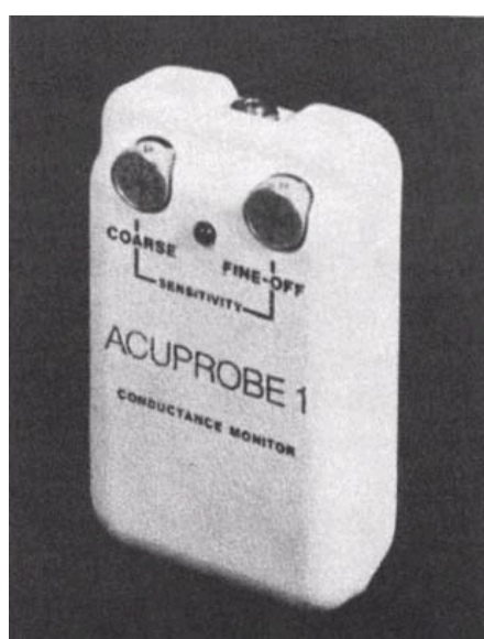
Figure 2-25. The Acuprobe I-a small, hand-held, unit for point location by skin conductance measurement, capable of sensing with very low currents in the region of 0.5-1.0 microamperes. Indication is by means of an audible sound plus a visual red light output. Probe-sensing is adjustable by means of two sensitivity controls, coarse and fine, for a full range of skin resistances. The power source is a standard 9-volt transistery battery. (Courtesy of Intertronic Systems, Ltd., Ontario, Canada.)
