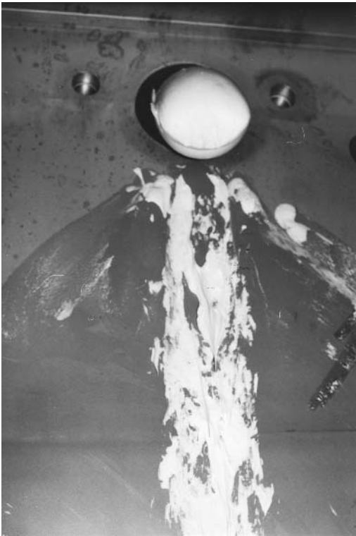
Figure 4 Butter is discharged into the covered silo.
