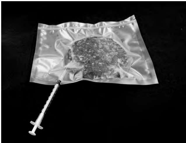
FIG. 4 Antimicrobial packaging of ground beef. The plastic pouch contains antimicrobial paper under the ground meat, which releases volatile antimicrobial agent (allyl isothiocyanate). The syringe takes headspace gas samples to monitor the effective concentration of the volatile antimicrobial agent inside the pouch to inactivate Escherichia coli O157:H7. (From Nadarajah et al., 2005b.)
