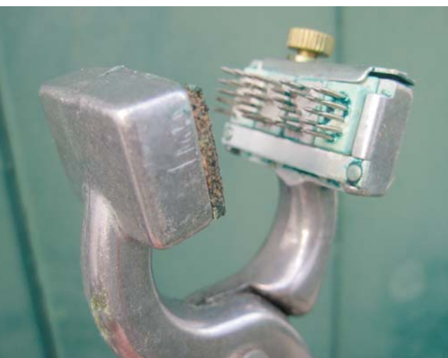
Tattoo pliers with symbols secured in place.
