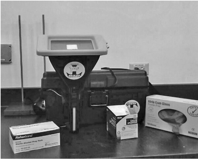
Figure 5.3 Scent Transfer Unit (STU-100) collection kit. (Photo courtesy of Claudia L. Sanchez.)
