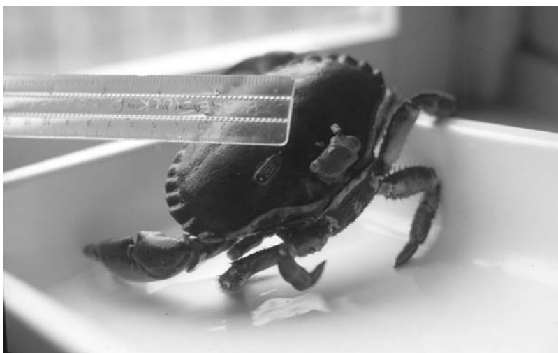
Figure 12.1 Ultrasonic heart-rate telemetry tag fitted to the carapace of Carcinus maenas during a procedure using no anaesthetic. The crab lived for many days before leaving the range of the receiving equipment. (L.G. Ross, unpublished data).
