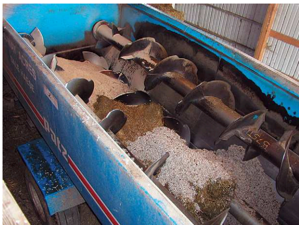
Figure 5-11 In this case the two screws on either side of the bin mix in opposite directions and the screw in the base performs the delivery. (Courtesy of K Nordlund)
