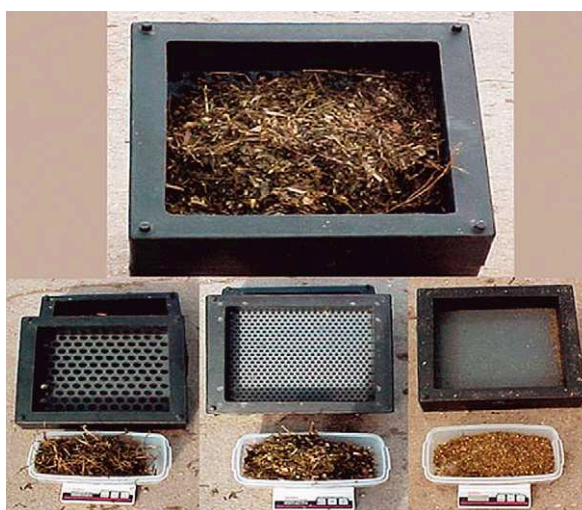
Figure 5-9 The Pennsylvania State Separator consists of three boxes and a pan. Between each box there is a sieve with holes decreasing in size. The material to be examined is placed on the uppermost filter and shaken from side to side 40 times. The boxes are rotated one-quarter turn every five shakes. The larger particles on the top screen will float in the rumen and require more chewing. The particles in the middle box will be digested more slowly, while those in the bottom box will be fermented rapidly and pass out of the rumen quite quickly. (Courtesy of R Shaver)
