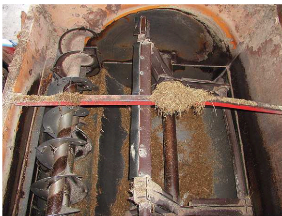
Figure 5-10 There are many designs of mechanical feed mixers. In this case a paddle does most of the mixing while the screw delivers the final mix. The efficiency of any mixer depends on the operator mixing consistently and according to the instructions of the manufacturer. (Courtesy of K Nordlund)
