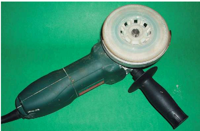
Figure 14-60 A small domestic angle grinder is suitable for use in claw trimming. (Courtesy of A Brizzi)
