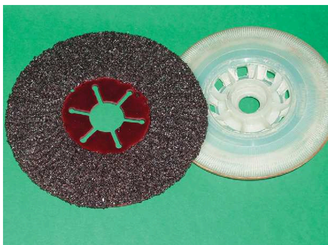
Figure 14-62 Fiber-backed grinding disks must also be supported by a synthetic backing disk. (Courtesy of A Brizzi)
