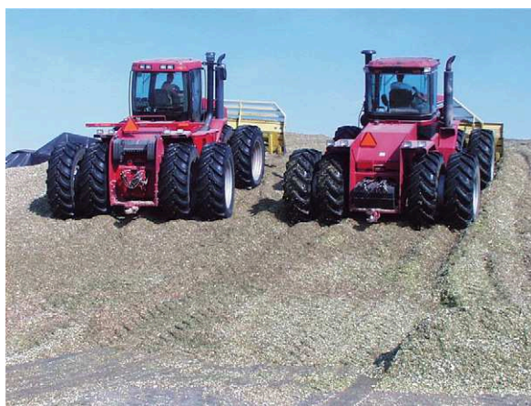
Figure 5-15 These heavy units compact the silage very effectively, reducing air pockets to a minimum. Good compression reduces the necessity for chopping the crop too small. Good particle size is essential for proper digestion. (Courtesy of K Nordlund)
