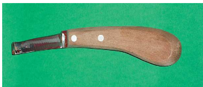
Figure 14-56 Swedish knives are perhaps the most popular in use at this time. They are noted for holding a sharp edge for longer than other makes of instrument. (Courtesy of A Brizzi)
