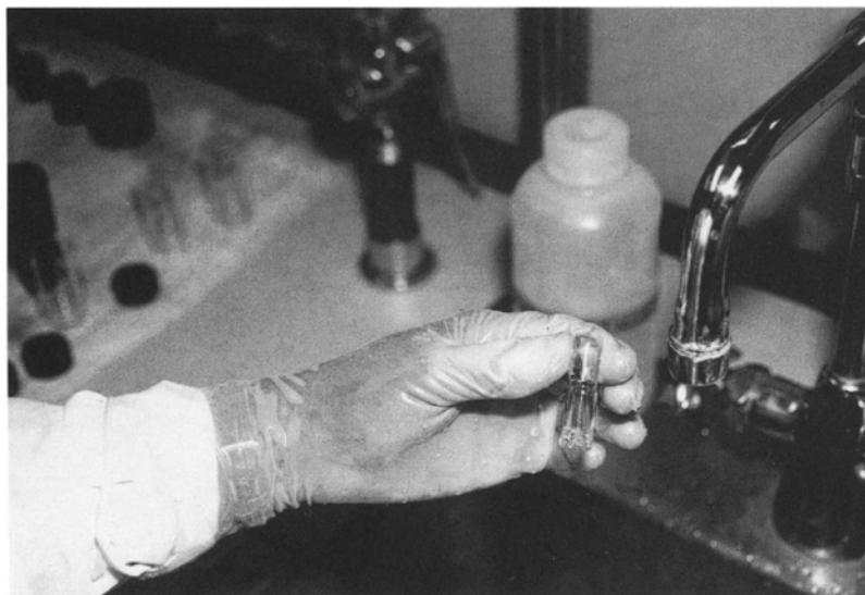
Figure 66. Ampule with recrystallized osmium in the bottom portion of the ampule.
