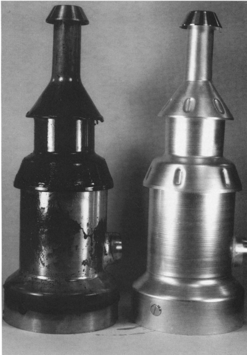
Figure 205. A diffusion stack with dark, oxidized (cracked) oil on its surface, next to a new diffusion stack with clean metal surfaces.
