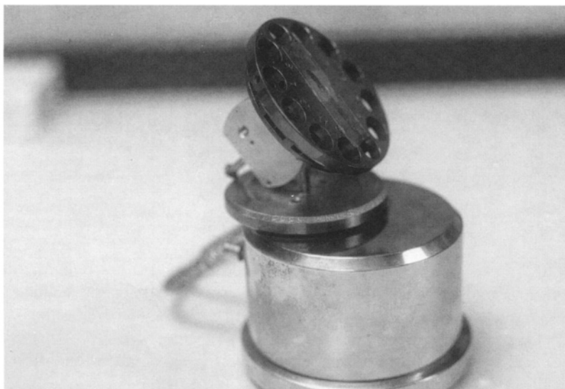
Figure 223. Specimen holder for coating SEM samples in a vacuum evaporator (from a Ladd Vacuum Evaporator).
