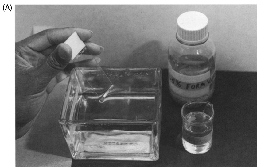
Figure 154. Stripping Formvar from a microscope slide. (A) Touching the slide to the water surface.
