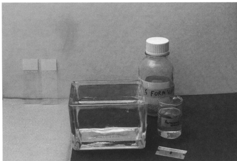
Figure 152. Formvar-coated microscope slides drying on a paper towel.
