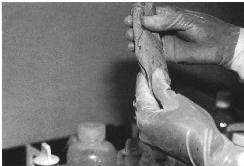
Figure 67. Ampule containing osmium wrapped in several layers of paper towels, ready to be snapped in two.
