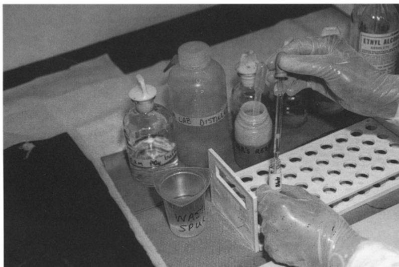
Figure 58. Removing resin from a sample vial with a glass 5\frac{1}{4} in. (13 cm) Pasteur pipet for transfer to waste Spurr resin beaker, shown to the left in the photo.
