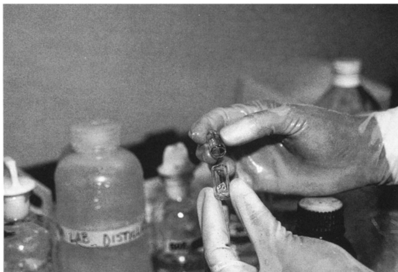
Figure 68. Ampule after breaking into two pieces, the bottom half containing osmium crystals.
