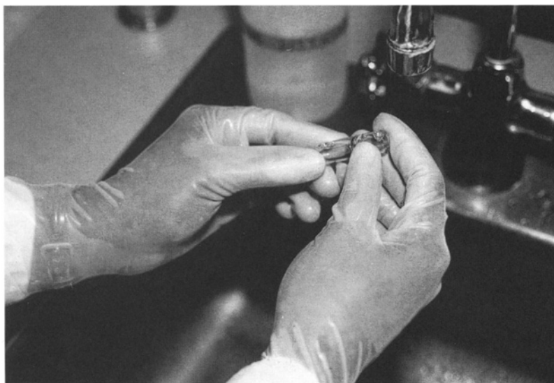
Figure 64. Osmium crystals in a sealed ampule, located both above and below the constricted and scored portion of the ampule, which will be the break line when the vial is snapped.
