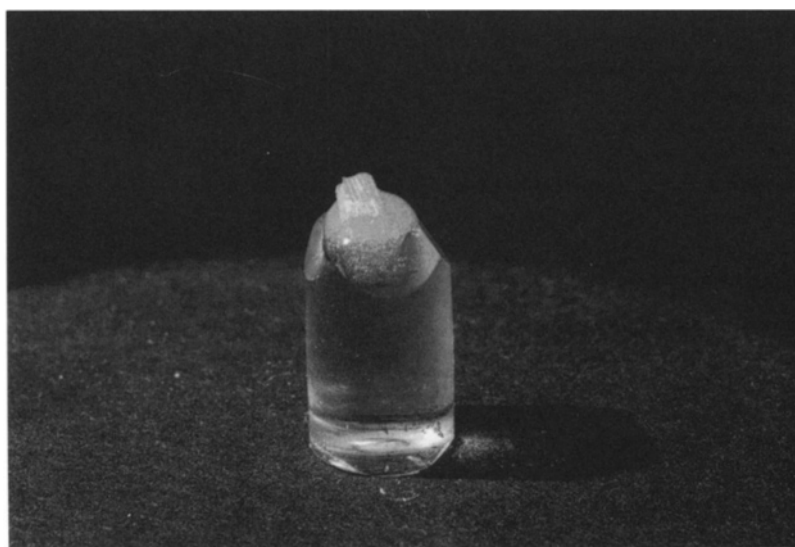
Figure 77. Embedded monolayer mounted on blank epoxy block with 5-min epoxy cement.
