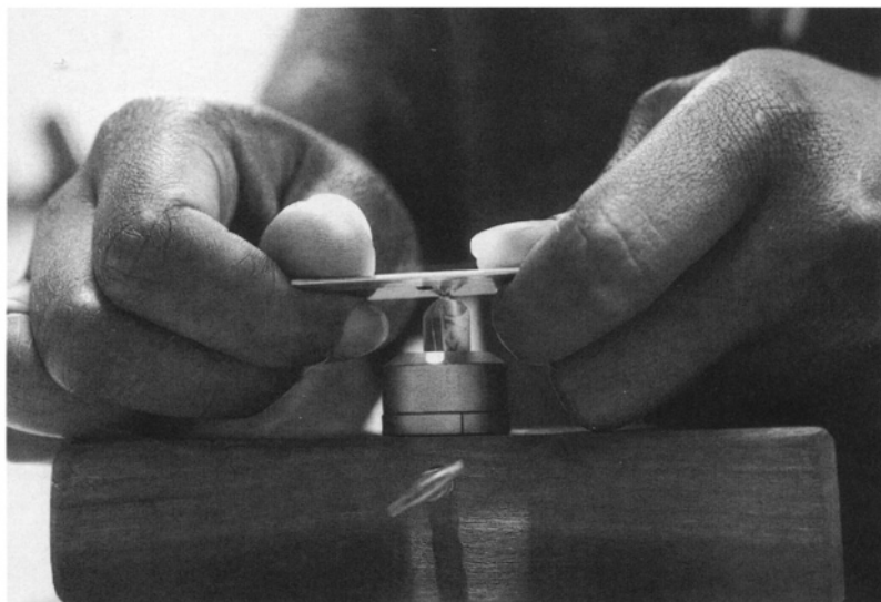
Figure 112. The safest method for holding a razor blade during block trimming. Note: Both hands are holding the razor blade to totally control the cut.
