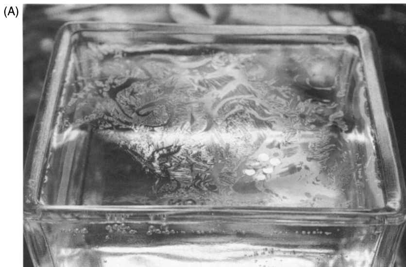
Figure 157. Film casting and grid retrieval as used with the droplet method (Parlodion). (A) The film created by dropping Parlodion solution on the surface of water in a slide-staining dish is wrinkled and variable in interference color. Note the grids placed on a relatively wrinkle-free area.
