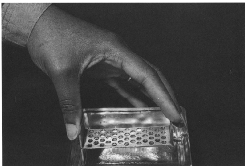
Figure 155. Aluminum bridge being touched to a Formvar film floating on water in a staining dish.
