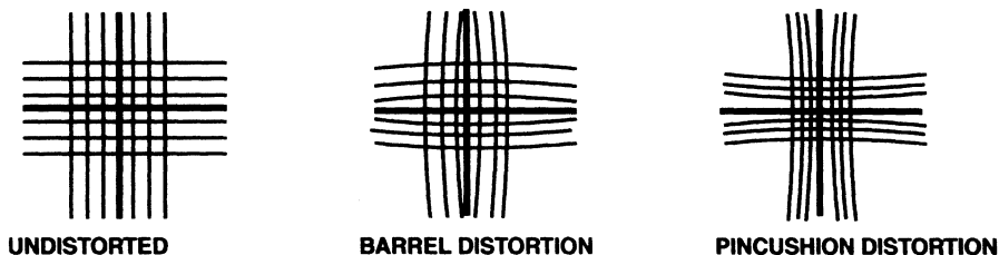
Figure 181. Undistorted image of a grid compared with barrel and pincushion distortion (spherical aberration).
