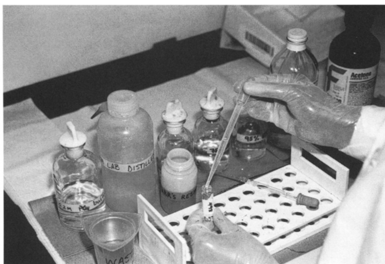
Figure 59. Adding Spurr resin to a sample vial with a plastic transfer pipet from a polypropylene bottle containing fresh resin, located behind the tube rack.
