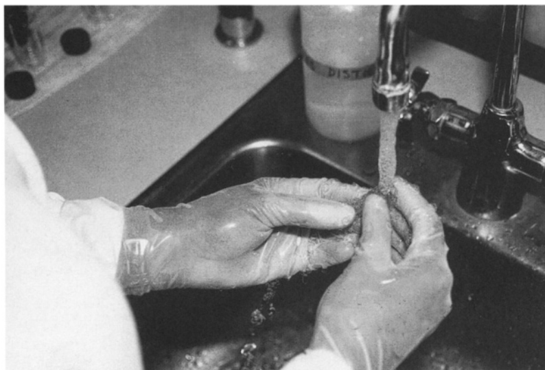
Figure 65. Running warm water over the ampule to melt the osmium crystals so that they will run into the bottom half of the ampule.
