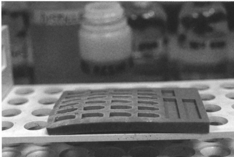
Figure 73. Silicone embedding mold used with Spurr resin. The mold has probably been used two dozen times and has interacted with the resin. The resin has caused the mold to curve. When the polymerized blocks were removed from the mold, small pieces of the silicone were pulled away, as can be seen in the corner of the chamber at the lower left.
