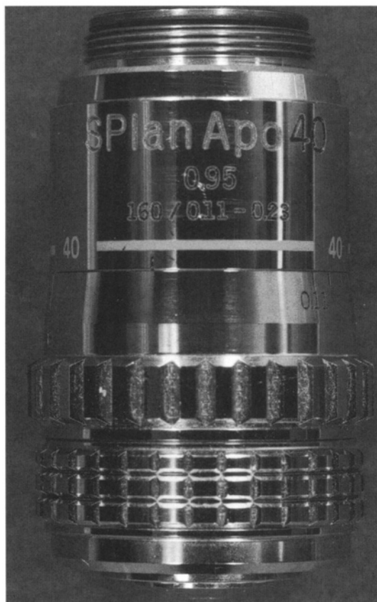
Figure 267. A flat-field 40 \times apochromat objective intended for use on a microscope with a 160-mm tube length. The numerical aperture of the lense is 0.95, and the high-dry lens may be used with #1, #1.5, and #2 coverglasses, as well as for specimens of various thickness. The focusing collar should be adjusted empirically for various specimens, until the image is as sharp as possible.
