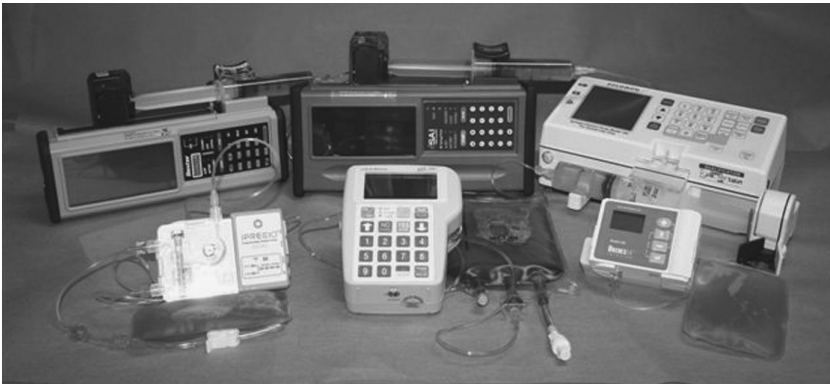
Figure 3.6 Various types of infusion pumps allow the researcher to accommodate different study designs. Newly designed infusion pumps are capable of wireless and/or Ethernet connectivity, allowing for remote pump monitoring and/or control.
