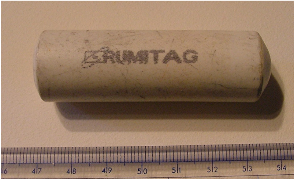
A ruminal bolus, a ceramic cylinder containing a transmitter by means of which animal identification is achieved
