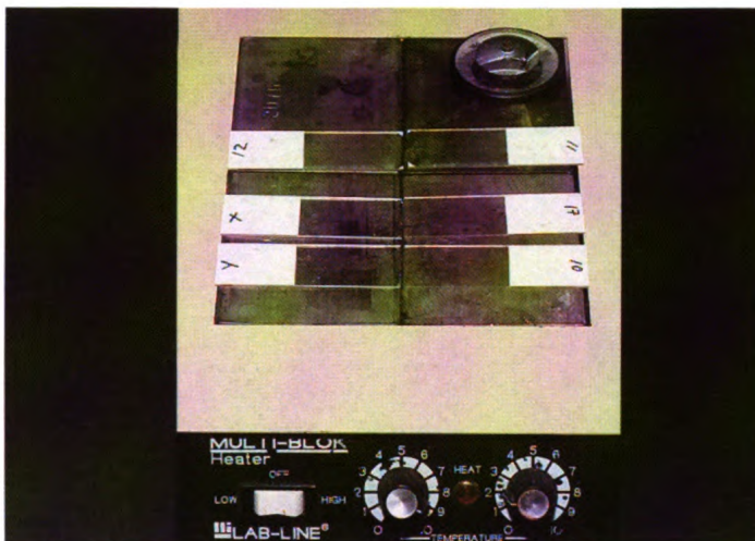
Fig. 2-9. Denaturing using dry heat block 98° to 100°C.
