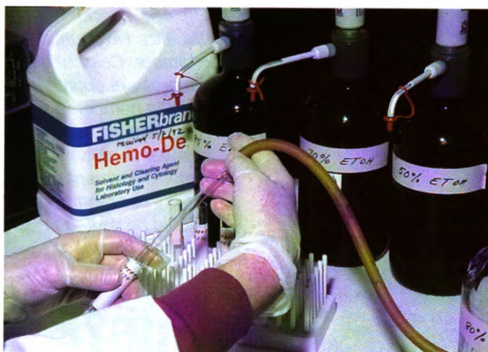
Fig. 4-3. Exchange of solutions by aspiration.
