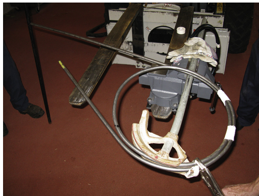
Fig. 1. A pipe bender is shown secured in a vise as used to bend 0.25-in steel bar to make the ring and proximal leg rods for the TSCC. A section of equine stomach tube was placed in the calf's axilla to determine the appropriate ring size and used as a template for bending the bar.
