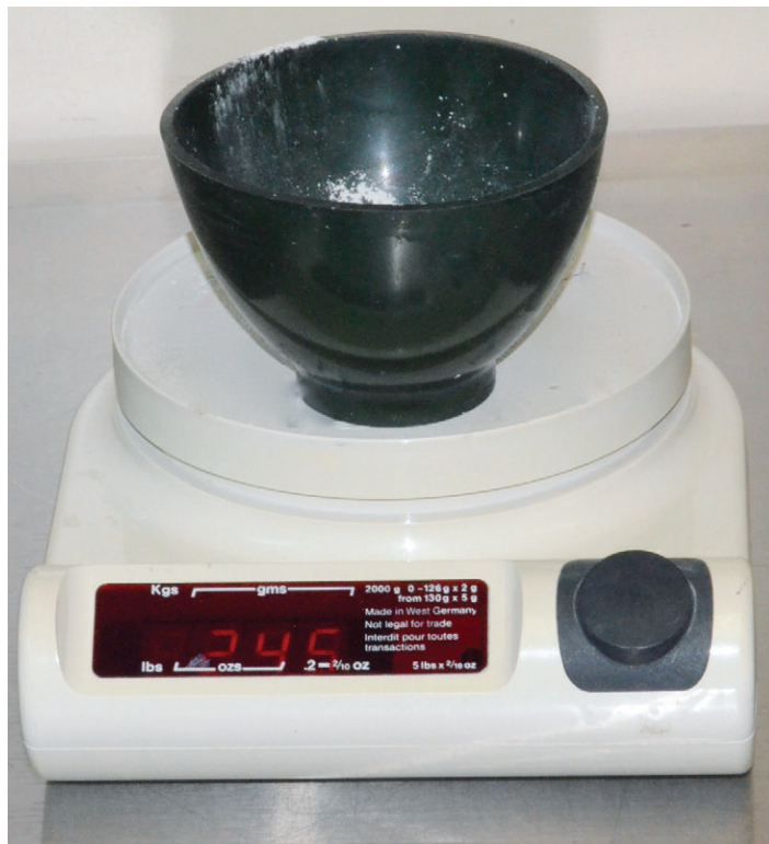
FIGURE 13-26: A gram scale is used to measure the powder portion of the dental stone.
