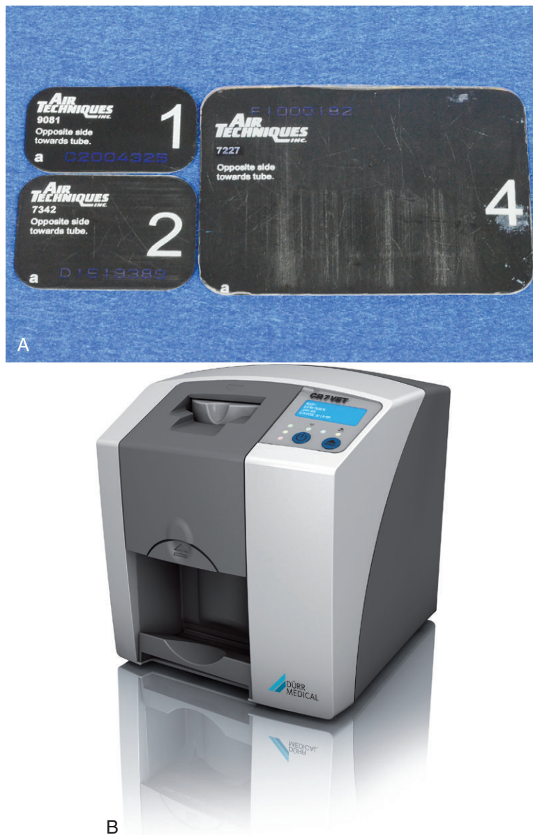
FIGURE 11-8: Plates (A) and processing unit (B) for computerized radiography (CR).
