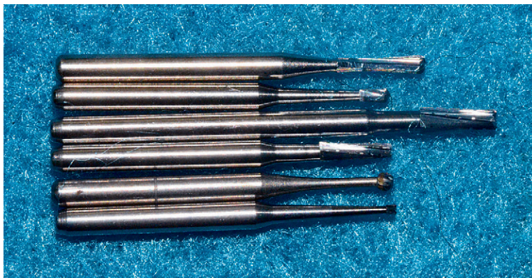
FIGURE 3-48: Top to bottom, 331 L (long pear), 330 (pear), 701S (surgical length), 701 (crosscut fissure), 2 (round), 33½ (inverted-cone bur).
