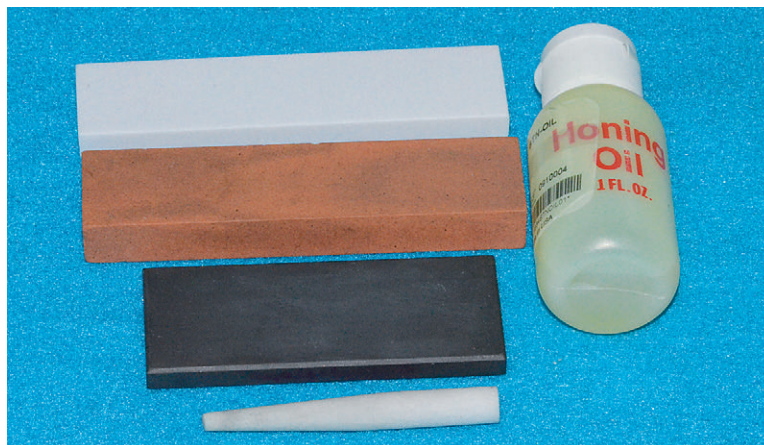
FIGURE 3-19: A variety of stones and oil is necessary to sharpen instruments. Top , Arkansas stone. Top middle , India stone. Lower middle , Ceramic stone. Bottom , Conical stone.
