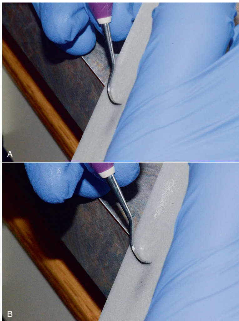
FIGURE 3-24: A , The instrument is placed so that the face is 90 degrees to the stone. B , It is then rotated outward 10 to 15 degrees.
