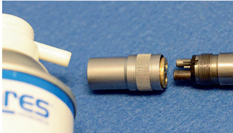
FIGURE 3-50: This system has a spray canister with lubricant and a connector that connects with the high-speed handpiece.
