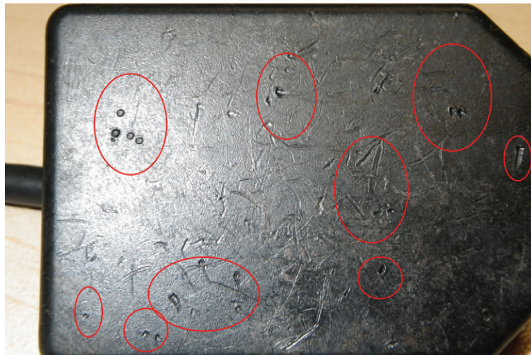
FIGURE 11-12: This sensor damage on the outside ( red circles ) may destroy the electronics inside.
