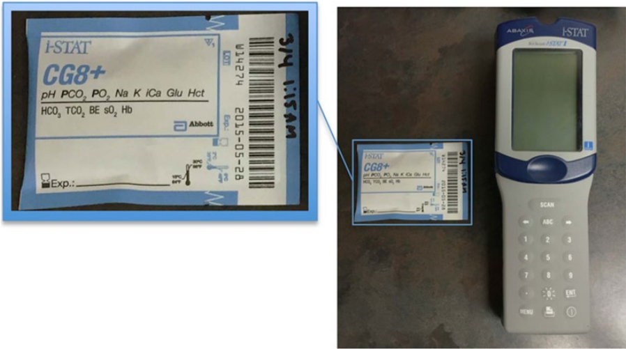
Figure 9.4 Abaxis I-Stat point-of-care blood gas analyzer and a CG8+ cartridge, which is a common device for obtaining quick and reliable blood gas values.
