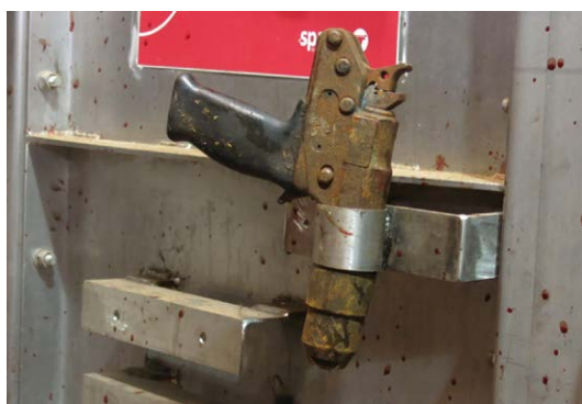
Fig. 12.6. Corroded captive bolt pistol, corrosion makes the machine less likely to be effective. (Image credit: Paul Whittington, AWT, 2017.)
