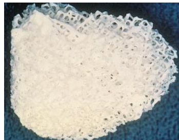
Fig. S28U: Overview of a porous cancellous Bio-Oss® block (left) and a close-up view, depicting the trabecular pattern of the sample (right).
