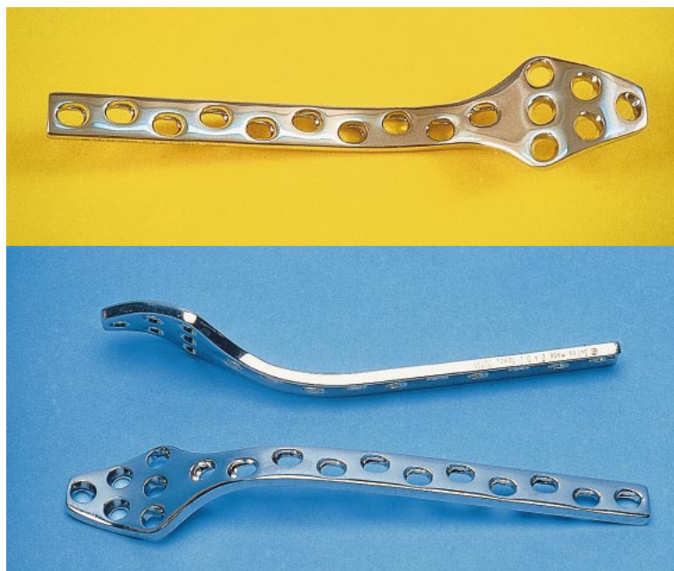
Fig. S14C: The cobra plate has six round holes in its “hood” that will accept 5.5–6.5 mm screws and allow angulation of about 15°. A good purchase can be achieved in short, thick fragments.
