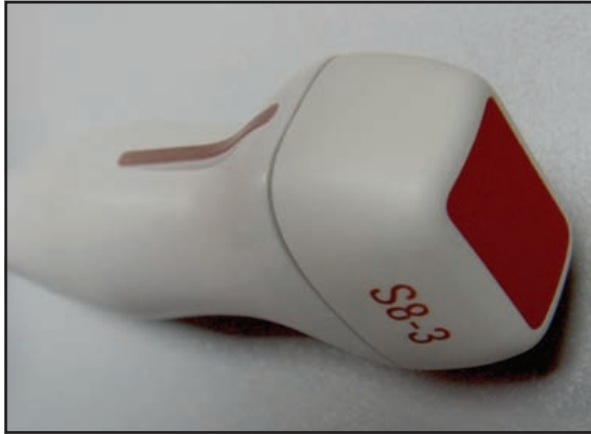
6.9 Phased-array transducer. The index mark on the transducer indicates the plane of the ultrasound beam.
