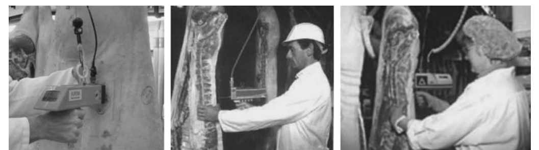
Figure 17.1 Different electronic probes: Hennessy Grading Probe (by Hennessy Grading System Ltd., with permission), CGM Probe (by Sydel, with permission), and Fat-O-Meter (by SFK Technologies, with permission).
