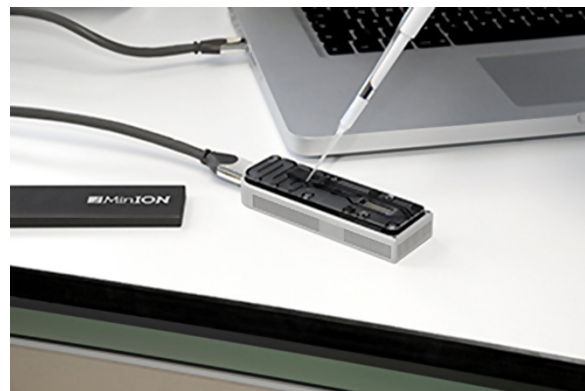
Figure 24.20 The MinION (Oxford Nanopore Technologies) plugs directly into a laptop or desktop computer through a USB port, and is a self-contained device to deliver real-time data. (Courtesy of Oxford Nanopore Technologies.)
