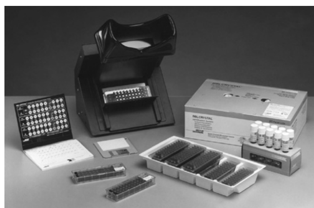
Figure 4.7 BBL Crystal ANR ID. Thirty wells in a plastic base are aligned and snapped together with a lid containing 29 biochemical and enzymatic substrates. Some reactions are visualized with a UV light reader (upper left center), while others are read and interpreted using ambient light. (Courtesy and © Becton, Dickinson and Company.)
