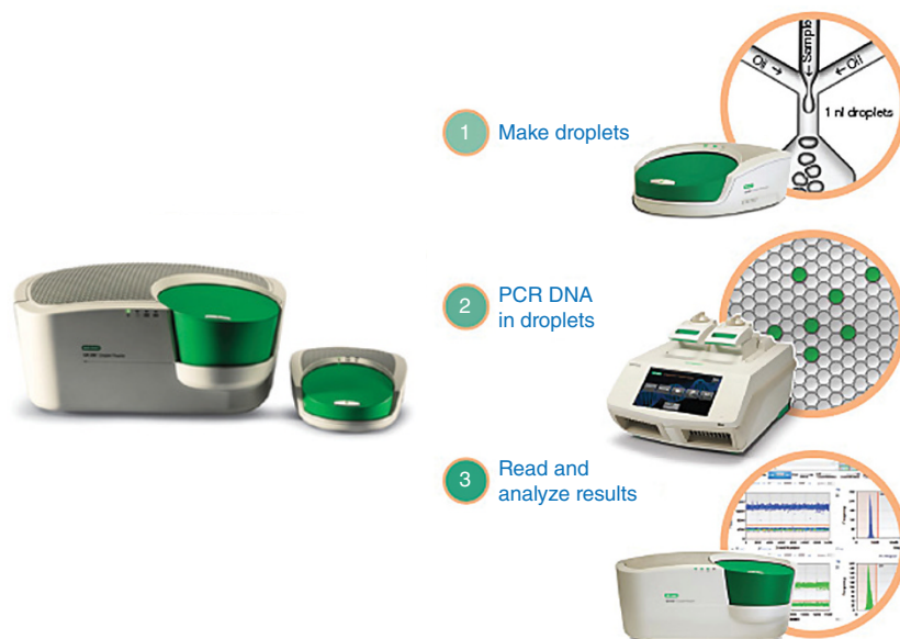
Figure 24.5 Bio-Rad's QX100 Droplet Digital PCR system (ddPCR) is a novel way to accomplish quantitative PCR. (Courtesy of Bio-Rad Laboratories, Inc.)
