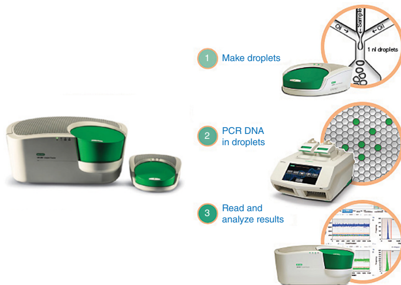
Figure 24.5 Bio-Rad's QX100 Droplet Digital PCR system (ddPCR) is a novel way to accomplish quantitative PCR. (Courtesy of Bio-Rad Laboratories, Inc.) (See insert for color representation of the figure.)
