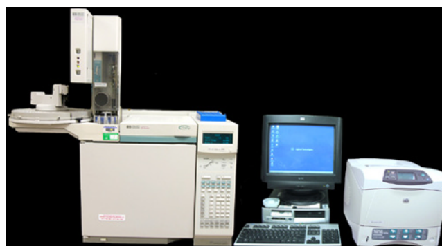
Figure 4.10 MIDI Sherlock Microbial Identification System, an automated GC analytical system. Included in the photograph are the following: an Agilent 6890 GC with an automatic sampler, a computer, and a printer. The GC contains a fused-silica capillary column and a flame ionization detector. (Courtesy of MIDI.)
