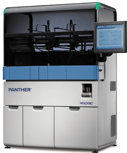
Figure 24.11 Hologic's PANTHER instrument tests ThinPrep liquid cytology specimens via Aptima HPV mRNA-based assay is a nucleic acid amplified test that detects 14 high-risk strains of human papillomavirus (HPV) associated with cervical cancer and precancerous lesions. (Courtesy of Hologic, Inc.)
