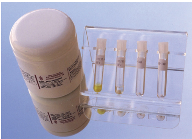
Figure 4.1 WEE-TABS stand-alone chromogenic tests. Each tube contains one tablet and a small volume of bacterial suspension. (Courtesy of Key Scientific Products.)
