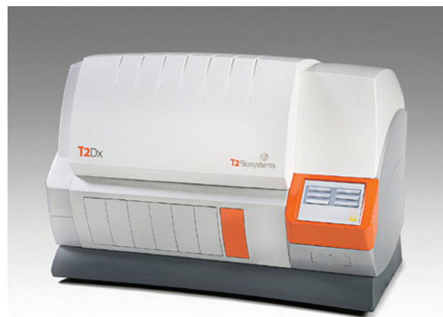
Figure 24.24 T2Dx Instrument from T2 Biosystems uses magnetic resonance for identification of microbes. (Courtesy of T2 Biosystems, Inc.)
