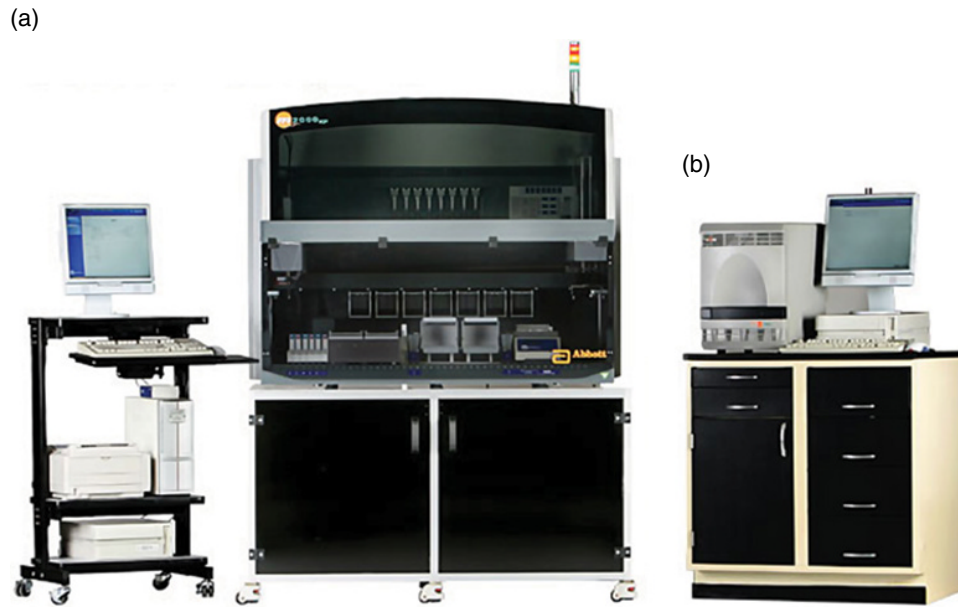
Figure 24.3 (a) Abbott's m2000 sp system for sample preparation is linked with (b) m2000rt for real-time amplification and detection to form a multicomponent system for qualitative and quantitative PCR and RT-PCR. (Courtesy of Abbott.)
