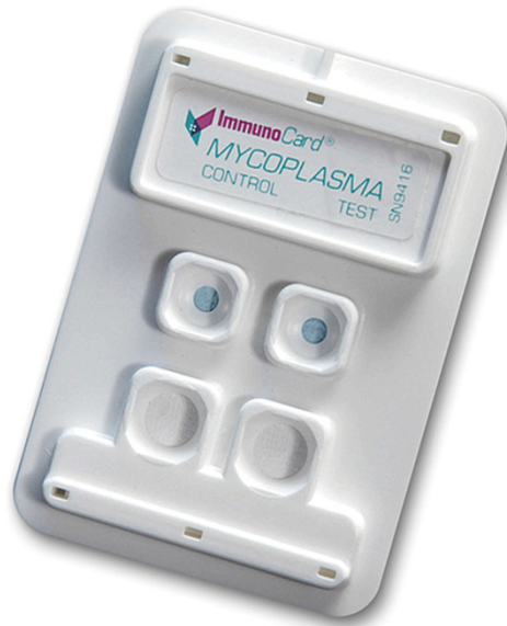
Figure 12.3 ImmunoCard (Meridian Bioscience, Inc.). The Meridian ImmunoCard is a qualitative, membrane-based EIA that can be performed in 10 min or less to detect the presence of IgM antibody directed against M. pneumoniae . A positive test is indicated by development of a blue color in both of the upper reaction ports. (Photograph courtesy of Meridian Bioscience, Inc.)
