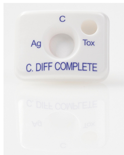
Figure 4.11 C. Diff Quik Chek Complete. This lateral flow rapid membrane enzyme immunoassay can detect C. difficile GDH antigen and toxins A and B simultaneously. (Photograph courtesy of Alere, Inc.)
