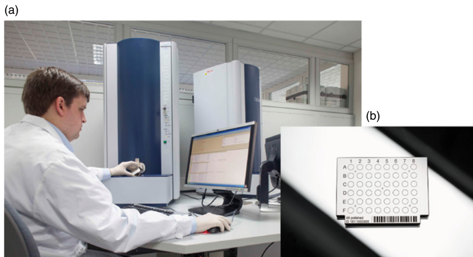
Figure 24.15 (a) The Bruker MALDI Biotyper CA System includes a bench-top microflex MALDI-ToF mass spectrometer, software, reagents, a library of microorganism reference spectra, and (b) a 48-spot MALDI target plate. (Courtesy of Bruker Daltonics.)
