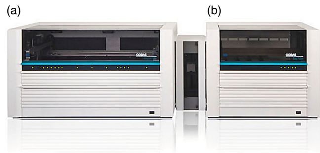
Figure 24.2 (a) The Roche COBAS system is comprised of the COBAS AmpliPrep instrument and (b) the COBAS TaqMan instrument. The two components are depicted here in “docked” mode, but can also be undocked and placed in separate laboratory areas. (Courtesy of Roche Diagnostics Corporation.)
