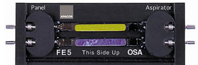
Figure 15.24 Detailed view (from Figure 15.23) of the glass viewing chamber that holds a portion of the concentration sediment and rests on the microscope stage. The fecal material is viewed through the microscope focused on the contents in the chamber. (Courtesy of Apacor Ltd USA, Brooklyn and New York.) (See insert for color representation of the figure.)
