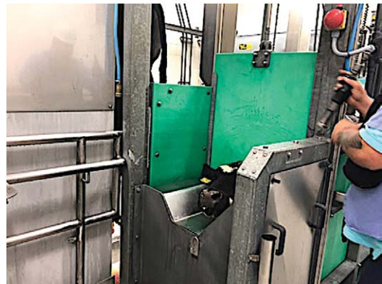
Fig. 6.1. The sliding panels that restrain the top of the bovine's neck and the box exit door are both constructed from thick plastic panels. This helps to reduce noise. (Photo courtesy of Temple Grandin.)
