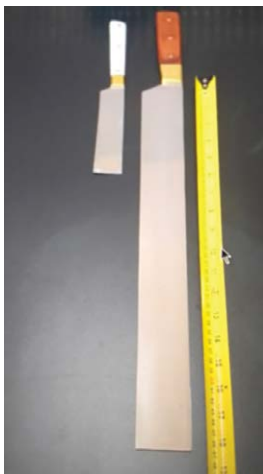
Fig. 11.9. Special long knives used for kosher slaughter. The use of a knife that is too short will cause gouging of the wound. It is the opinion of both authors that these are the only type of knife that should be used on adult cattle. (Photo courtesy of Erika Voogd.)
