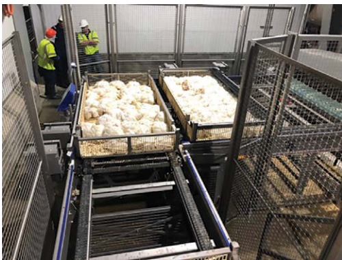
Fig. 8.2. Two decks from a stacked deck module system exiting the CAS stunning and moving towards the shackle system. (Photo courtesy of Temple Grandin.)
