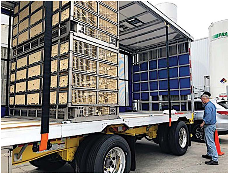
Fig. 8.1. An assembled four-deck stacked module that has been placed in the curtain-sided transport trailer. (Photo courtesy of Temple Grandin.)
