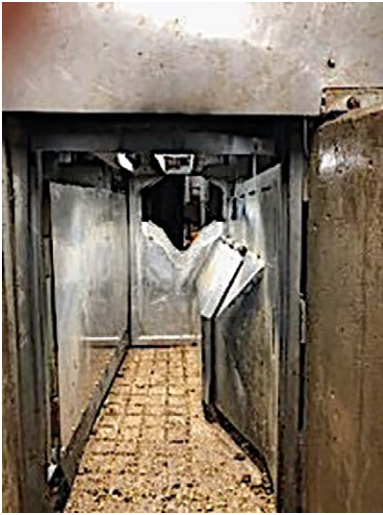
Fig. 6.2. Cow's-eye view into a stun box with a head yoke. Note the reflections on the shiny metal. Moving a ceiling light may eliminate these reflections. Make sure that an approaching animal does not see people through the head yoke. This stun box has a good non-slip floor. (Photo courtesy of Temple Grandin.)
