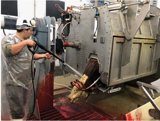
Fig. 11.6. Rotating box for cattle which holds two cattle. When one animal is in the inverted position, another animal is entering on the other side. The system rotates around a central pivot. Slaughter is conducted promptly after rotation. The vocalization score of approximately 20 Hereford cows was 0%. Washing the throat with the hose may increase stress and increases the length of time that the animal is restrained. (Photo courtesy of Temple Grandin.)
