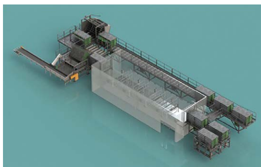
Fig. 8.4. Biphasic – Controlled atmosphere Biphasic stunning system. Marek Stork poultry – Processing patent 10085459b2. (Diagram courtesy of Humane-Aire, Bright Coop.)
