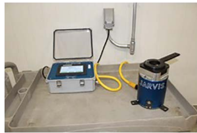
Fig. 10.8. A Jarvis brand hand-held captive bolt gun testing station. (Courtesy of Dennis William Willson.)
