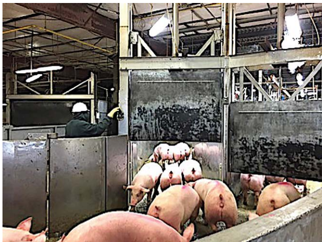
Fig. 6.12. Vertical slide gates constructed from flexible curtains made from conveyor belting will not injure the pigs if they are accidentally closed on them. (Photo courtesy of Temple Grandin.)
