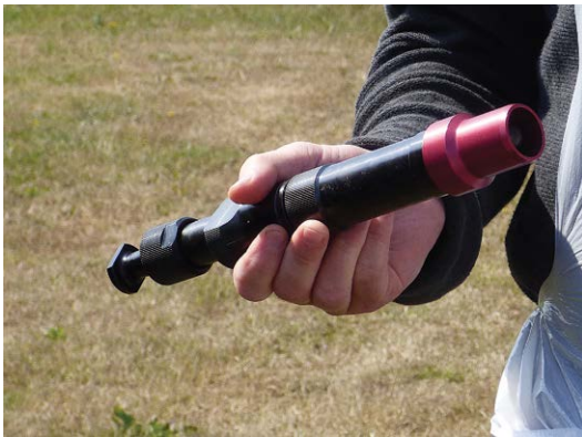
Fig. 7.5. An example of a cartridge-powered captive bolt gun for any size and type of poultry. (Photo courtesy of C. Berg.)
