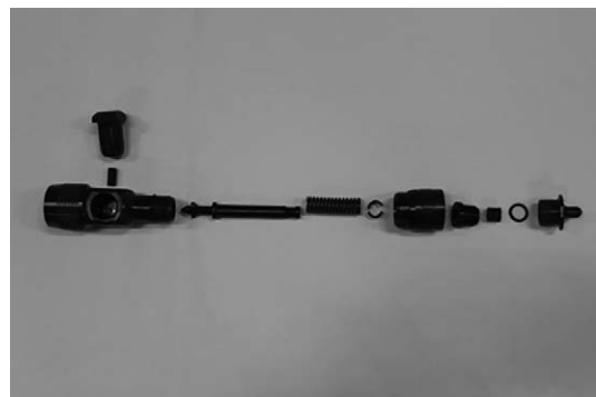
Fig. 10.4. Disassembled cartridge-fired in-line captive bolt gun. (Courtesy of Dennis William Willson.)
