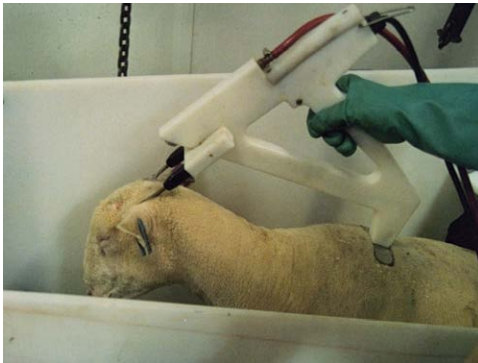
Fig. 9.2. Head-to-back cardiac arrest electrical stunning. It simultaneously induces unconsciousness and cardiac arrest. (From T. Grandin, 2010.)
