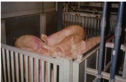
Fig. 9.6. A group of pigs getting ready to enter the CO 2 stunner. After the gate on the left side opens, the powered pusher gate on the right will move the pigs into the gondola. Group handling greatly reduces pre-stunning stress. (Photo courtesy of Temple Grandin.)
