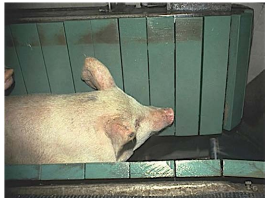
Fig. 6.14. V conveyor restrainer for either pigs or sheep. The slats are constructed from insulating plastic for use with electrical stunning of either pigs or sheep. Both sides of the conveyor must run at the same speed to prevent animals from struggling. Photo courtesy of Temple Grandin.
