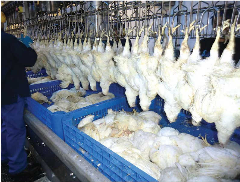
Fig. 7.7. The shackling station at a multi-stage carbon dioxide system where the birds are stunned in their transport containers and shackled after becoming unconscious. (Photo courtesy of C. Berg.)
