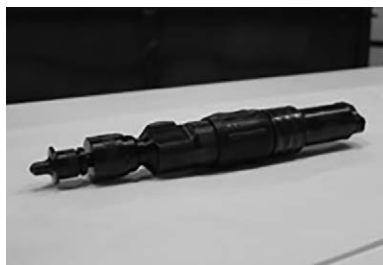
Fig. 10.2. A hand-held in-line penetrating captive bolt gun. (Photo courtesy of Dennis William Willson.)
