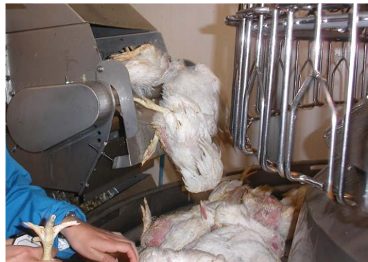
Fig. 7.6. A type of carbon dioxide stunning system where birds are first removed from the transport container, then taken on a conveyor belt through the two-stage carbon dioxide system, and finally shackled when unconscious. (Photo courtesy of C. Berg.)
