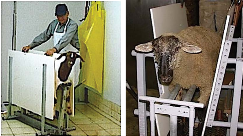
Fig. 11.4. Small restrainer for holding sheep or goats that is easy to build, based on a design by Westervelt et al. , 1976. (Photo courtesy of Spirit of Humane, Joe Regenstein.)
