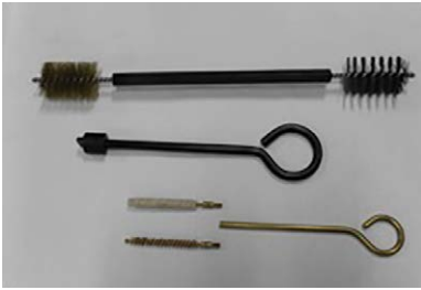
Fig. 10.6. An example of cleaning tools that can be used to regularly clean and maintain a captive bolt gun. (Courtesy of Dennis William Willson.)
