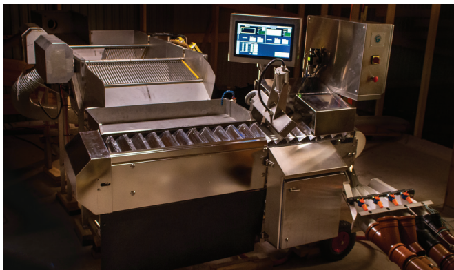
Fig. 21.1 A semiautomatic fish vaccination machine. Back left in the picture is the holding tank and anesthetic bath where the fish are brought in before vaccination. The sedated fish are then emptied on to the vaccination table where an operator places each fish, head down and belly to the left, in the trays of the transporter belt taking the fish to the vaccination station on the right. Every fish is photographed and a computer program tells the machine where to place the injection point. How far from the nose and how deep the injection is placed depends on the fish size. The fish data can be transferred to other computer units for later use and analysis. After vaccination the fish are sorted into three different sizes that have been set by the machine operator. Front right on the picture. One of the sorting stations is used for rejected fish, that is fish that are either too small or placed the wrong way onto the belt. The machine can vaccinate unsorted fish from 10 grams to 250 grams. Software that makes the machine suitable for specific species such as salmon, trout, sea bass, and tilapia has been developed. (Courtesy PHARMAQ Fishteq AS.)
