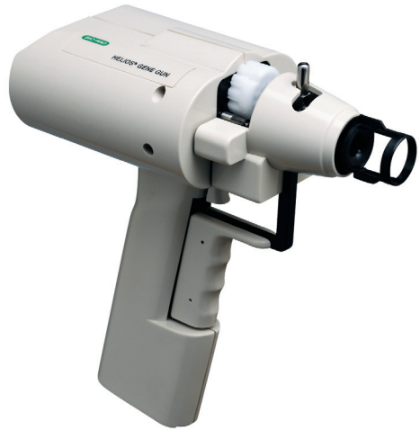
Fig. 6.3 A Helios gene gun. It uses a low-pressure pulse of helium to sweep DNA, RNA, or protein-coated gold particles from the inner wall of a small plastic cartridge directly into target cells. (From Bio-Rad Inc. With permission.)
