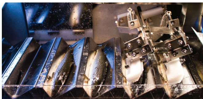
Fig. 21.2 Correctly placed salmon smolts in the fish trays of the transporter belt. A machine vision (photo technology) records their size and decides where to place the vaccine injection. Clamps gently hold the fish in place while the vaccine is injected, two fish are injected simultaneously in tray “one” and “two.” (Courtesy PHARMAQ Fishteq AS.)
