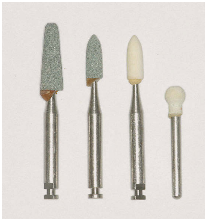
► Fig. 4.16 Finishing burs. After the tooth substance has been contoured, a finishing bur is used to smooth any edges that have been created and remove any enamel fragments. Green stones are used for more rough finishing and white stones (Arkansas) produce a smoother surface. Here too, various shapes are available.
