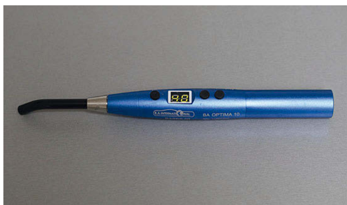
► Fig. 4.5 Curing light. A curing light enables use of composites with photoinitiators to create directly cured fillings. With an average 20-second curing cycle the part of the filling that has been inserted can be cured. The advantage of using materials cured by halogen light is that the pliable material can be applied and modeled until the result is satisfactory, while purely chemically cured two-component paste materials can only be handled for a limited time period.
