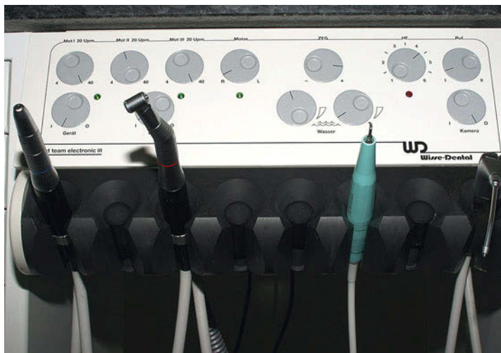
► Fig. 4.1 Dental unit. The basic prerequisite for performing comprehensive dentistry is a veterinary dental unit. To operate the rotary instruments, devices for holding the contra-angle handpieces and turbines are required. Another necessary item is a multifunctional syringe for spraying the working area with water or for drying it with air. An ultrasonic tooth scaler, a curing light, a high-frequency radiography machine or a suction device may also be integrated. Most veterinary dental devices offer a variable range of features.
