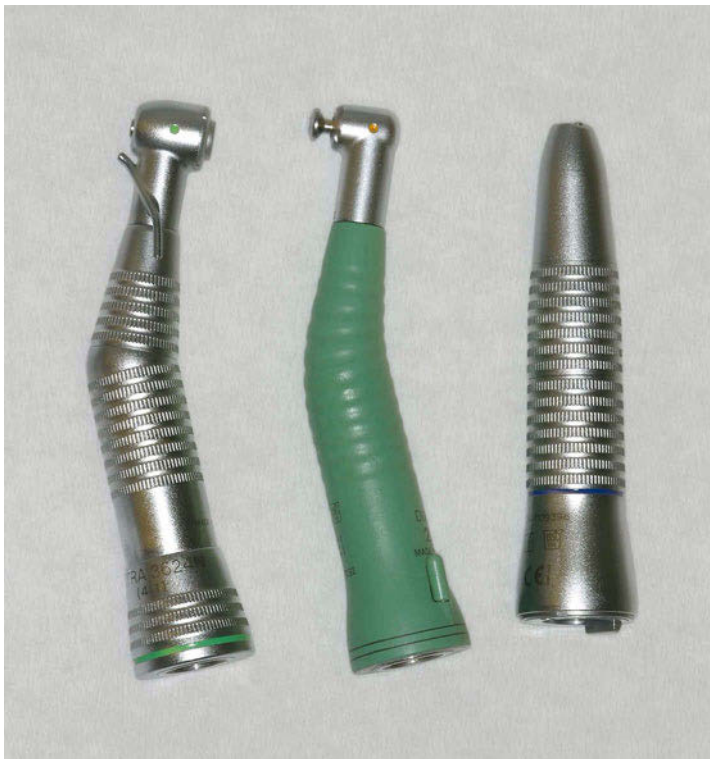
► Fig. 4.8 Special contra-angle handpieces and technical handpiece. Special contra-angle handpieces are available for special applications. On the left, a slow-speed surgical contra-angle handpiece is depicted with external water flow to the connection of sterile water coolant. The handpiece covered in green plastic has a holder for polishing cups. This handpiece is specially developed for polishing and prevents toothpaste from entering the head of the handpiece. On the right is a straight handpiece that holds rotary instruments for treating small domestic animals such as rabbits, guinea pigs, and chinchillas.
