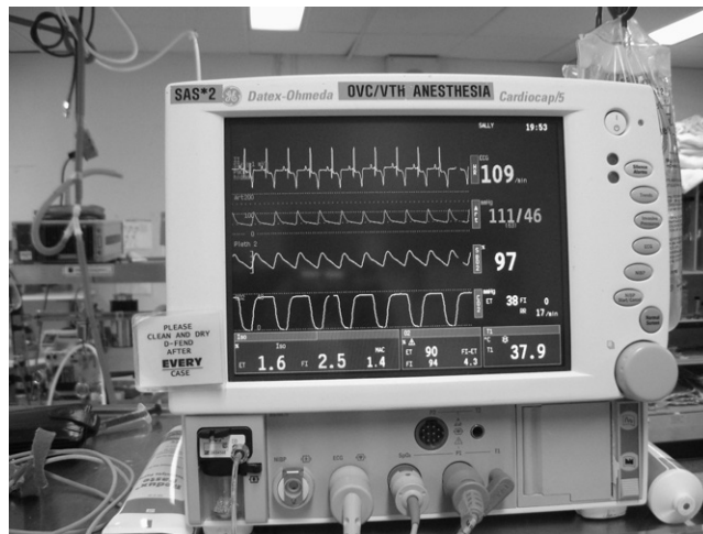
Figure 6.20. The waveform of the direct arterial pressure is second down from the top. The blood pressure measurement is read at the right side. Note that each wave spike in the arterial pressure corresponds with a complex on the ECG (an increase in pressure follows each contraction).
