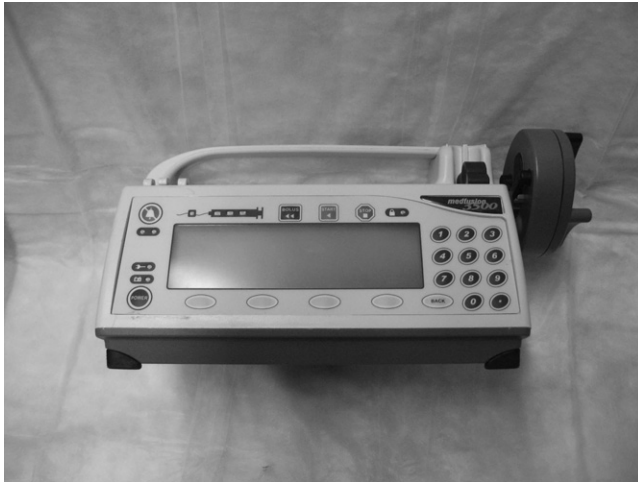
Figure 4.13. Syringe drivers can be used to deliver constant rates of infusions of medications or for single doses that are delivered over shorter periods of time.
