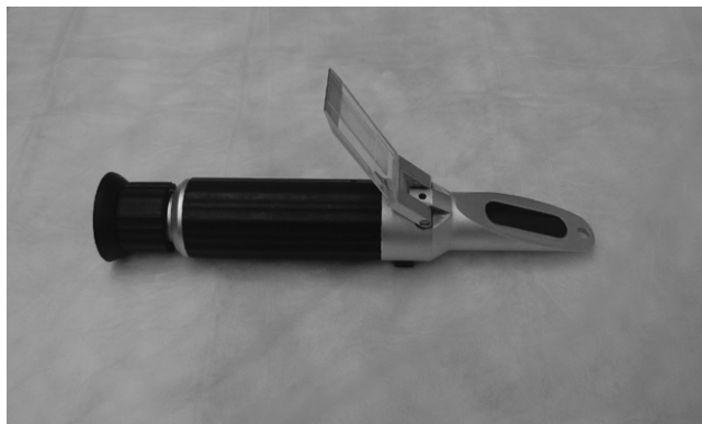
Figure 2.10. A refractometer is used to measure urine specific gravity.
