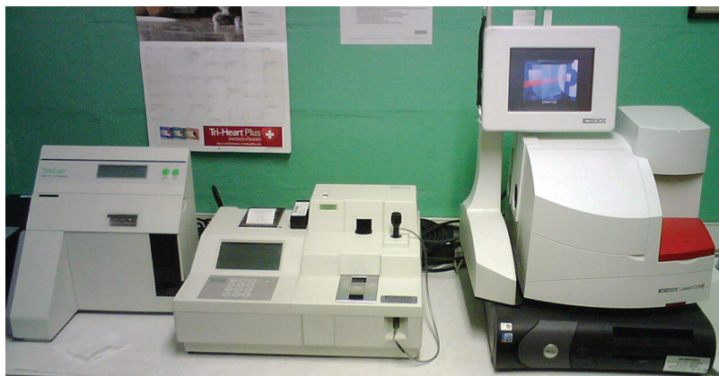
Figure 7.1 Bench-top automated hematology, electrolyte, and biochemistry analyzers used at small animal veterinary hospital.
