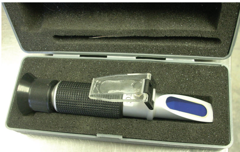
Figure 6.10 Clinical refractometer (TS meter).
