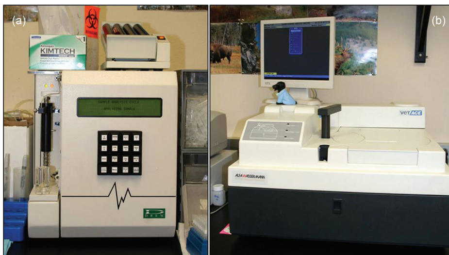
Figure 7.2 Bench-top automated hematology (a), electrolyte, and biochemistry (b) analyzers used at state veterinary diagnostic laboratory.
