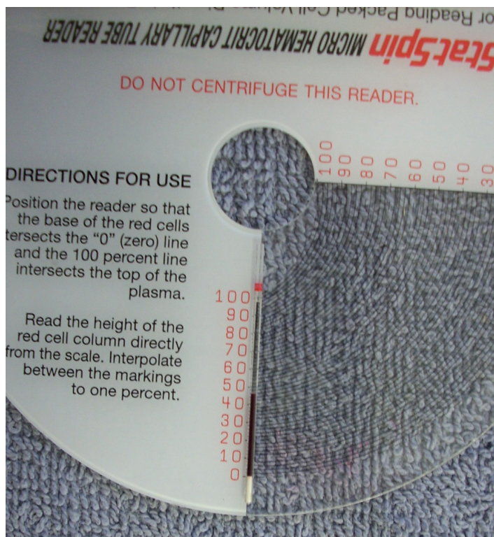
Figure 6.5 Measuring the PCV on a circular type of reader. Careful placement of the bottom of the blood column at “0” and the top at “100” is necessary for accurate measurement. This sample has a PCV reading of 46%.
