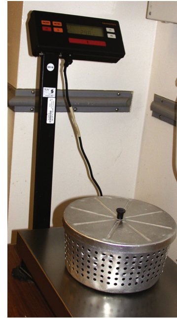
FIGURE 4.16 Weighing the patient is a vital part of monitoring health status. The scale should be able to read to \pm 1 g. (From Sirois M. Principles and practice of veterinary technology . 3rd ed. St. Louis: Mosby; 2011.)
