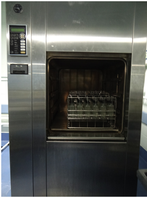
FIGURE 3.2 Small cages and racks of water bottles can be cleaned in this industrial washer.
