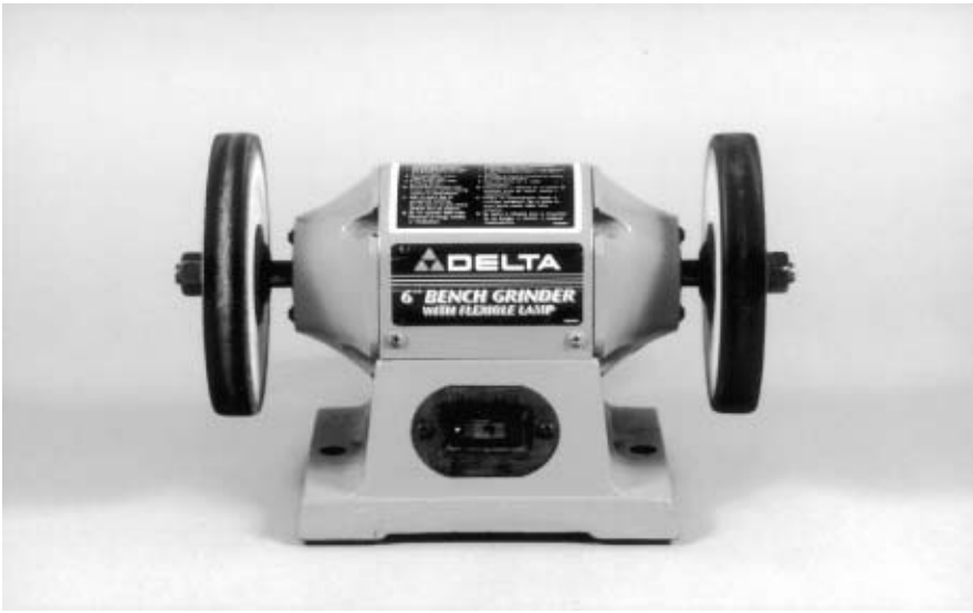
Figure 10.5. Bench grinder fitted with sharpening and buffing wheels.
