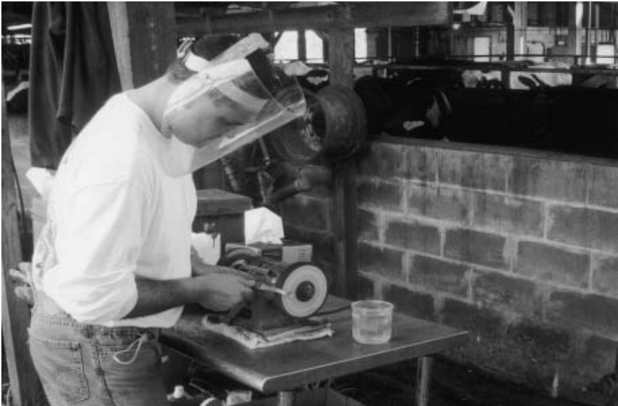
Figure 10.6. The wheels should rotate away from the operator.
