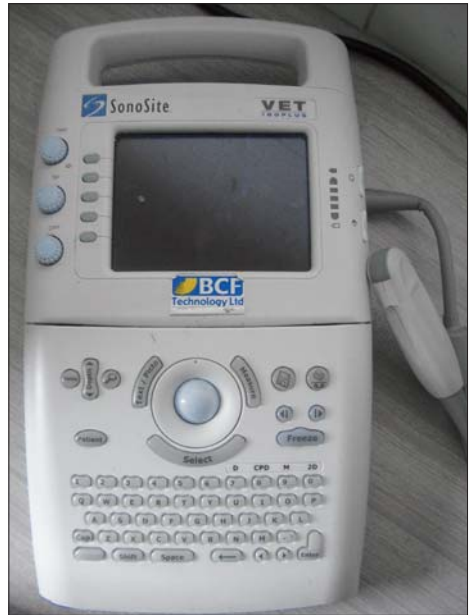
179 Ultrasound scanner and probe (5–10 MHz) typically available in general veterinary practice.
