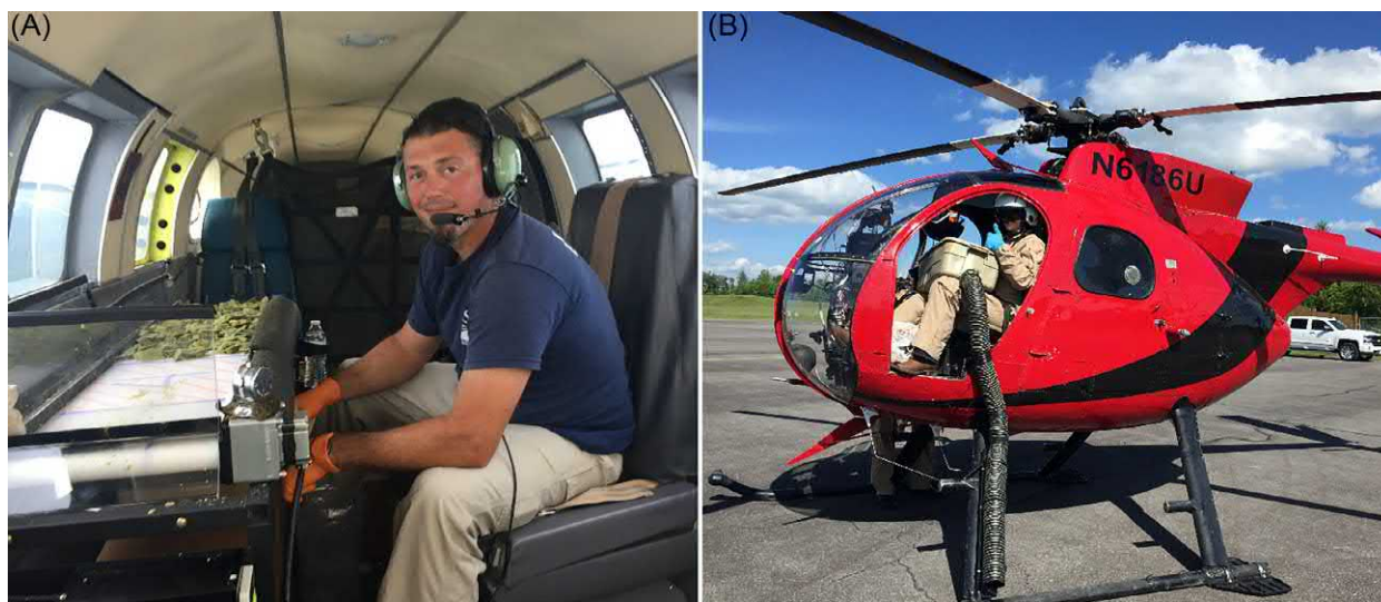
FIG. 19.7 Current machinery for distribution of oral rabies vaccine baits in the United States: (A) fixed-wing aircraft bait belt; (B) helicopter vacuum slide. Photos by USDA.
