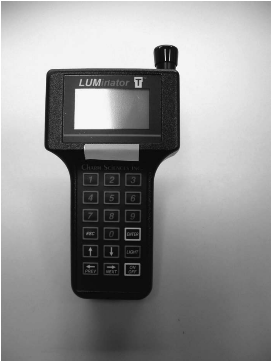
Figure 2.18 Lum-T meters (Charm Sciences, Inc., Malden, MA) are used to monitor for microbiological growth. Swabs are taken from equipment or room surfaces and inserted in a Lum-T meter, which instantly measures the presence of ATP.
