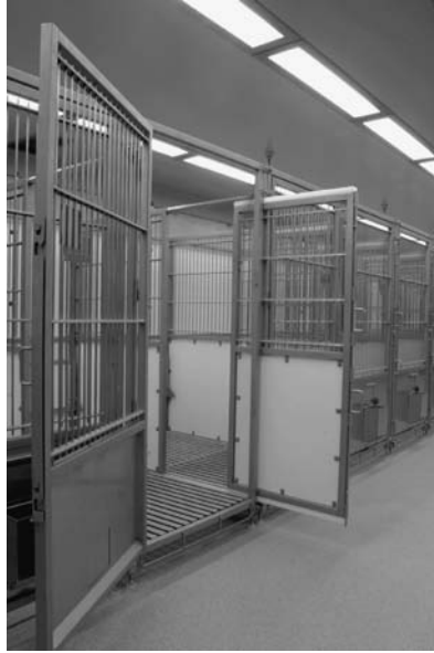
Figure 2.5 A dog kennel with an invertible/removable divider permits no contact (solid panel side down), moderate contact (gridded panel side down), or full contact (remove divider) between dogs. Note also the slatted flooring surface in the kennel. (Courtesy of Kevin Johnson, Allentown Incorporated)
