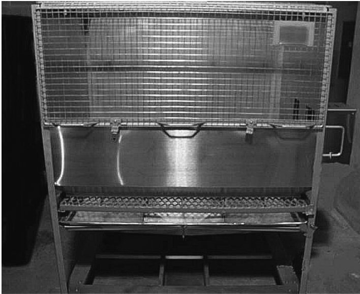
Figure 2.4 Metabolism cages are designed to permit collection of feces and urine during absorption, distribution, metabolism, and excretion (ADME) or pharmacokinetic studies. Often radioisotopes are used to label the test article for easier analyses.
