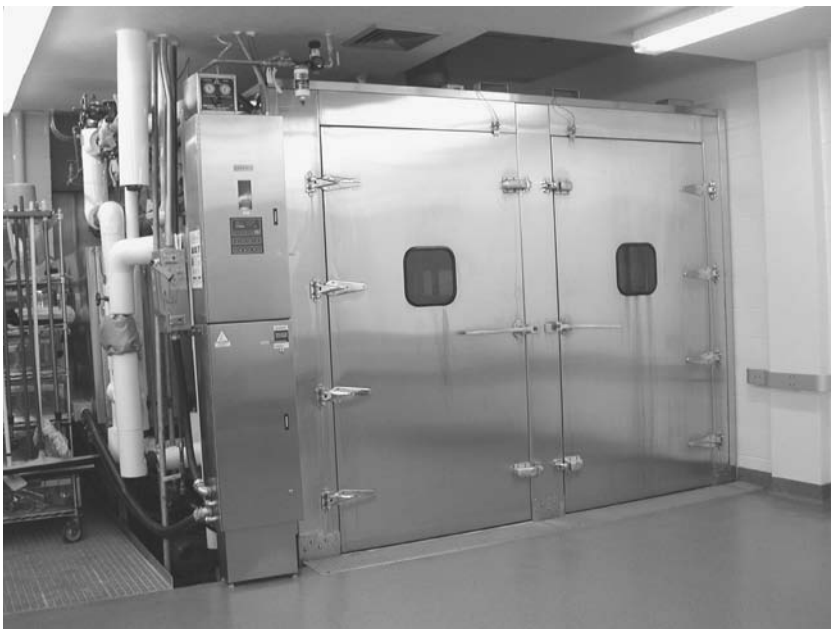
Figure 2.15 A mechanical rack and cage washer is a mainstay for sanitation of caging equipment. Time, temperature (including 180°F final rinse guarantee), and a variety of chemicals are used to ensure sanitation.
