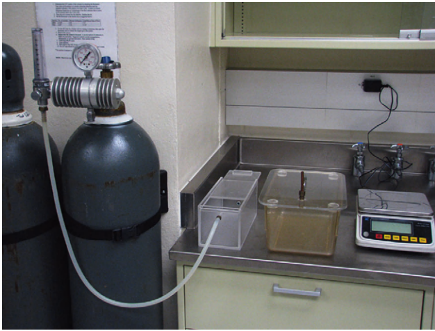
FIGURE 4.1 Example of CO 2 chambers and CO 2 tank with regulator valve.
