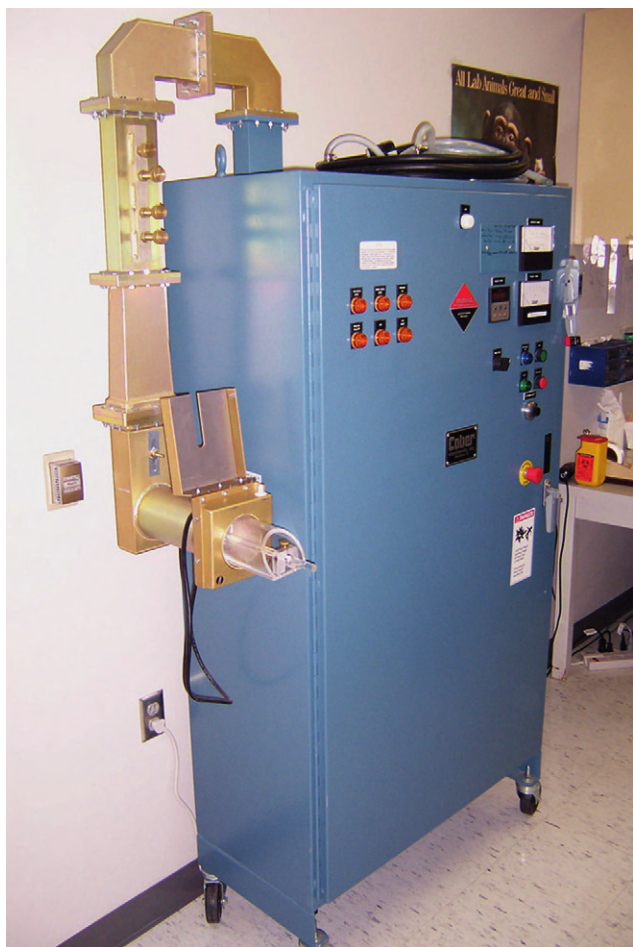
FIGURE 4.3 Microwave instrument used for euthanasia. Photo courtesy of Dr. Jonathan Geiger at The University of North Dakota, School of Medicine and Health Sciences.
