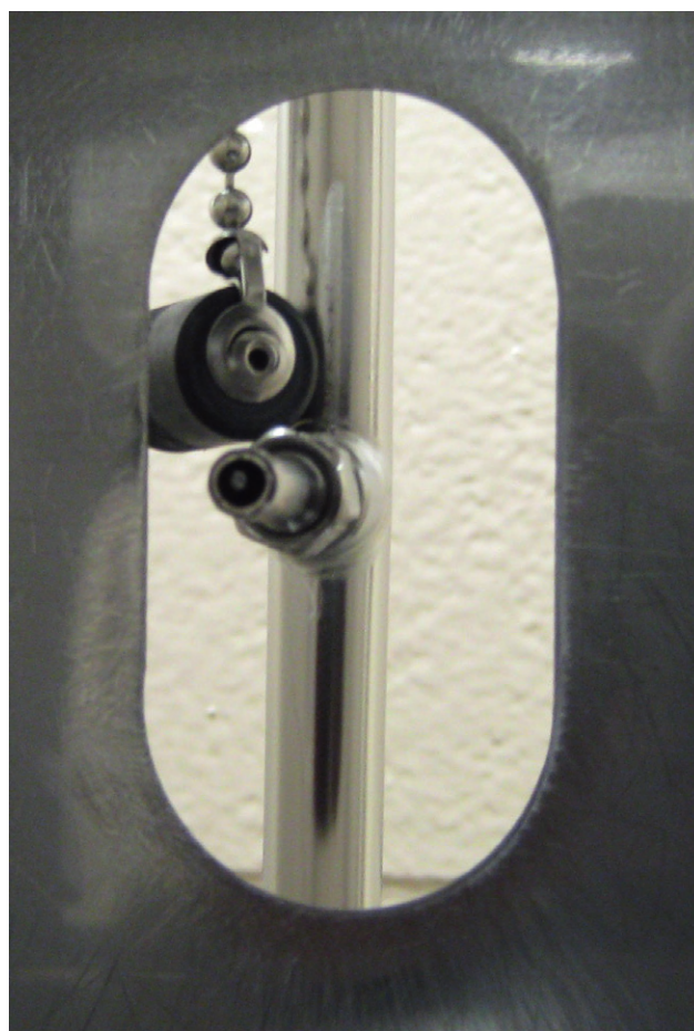
FIGURE 9.4 Automatic water drinking valve.
