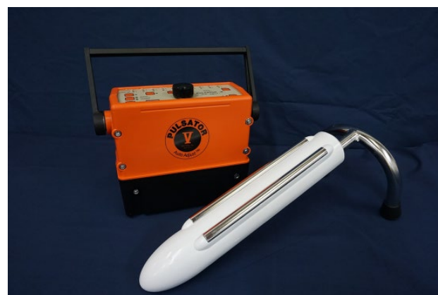
Figure 9.1 Lane Pulsator V and two-electrode probe with vertical yoke. Source: Courtesy of Lane Manufacturing, Inc.
