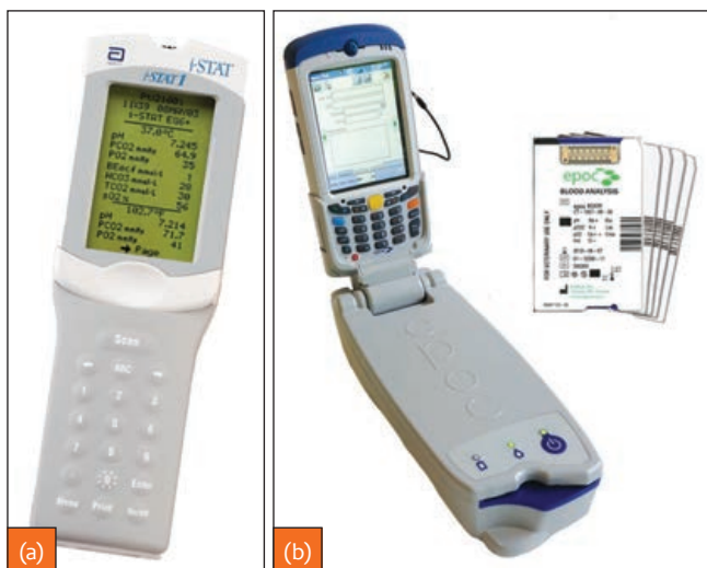
9.4 Two examples of hand-held blood gas analysers. (Courtesy of Woodley Equipment Company Limited)
