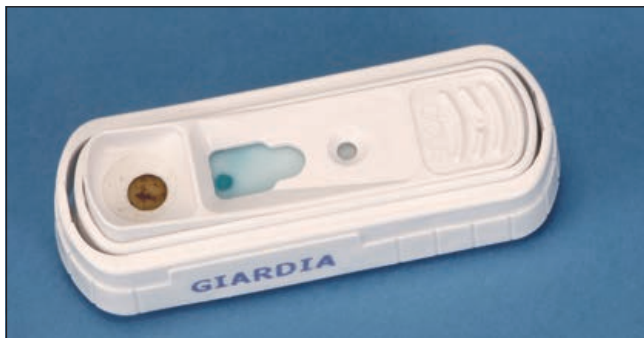
13.21 SNAP® immunochromatographic test for in-house testing for Giardia infection.
