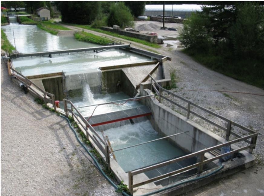
**Fig. 4.69** Prototype of a shaft power plant at the hydraulic field laboratory at Oberrach (P. Rutschmann)
