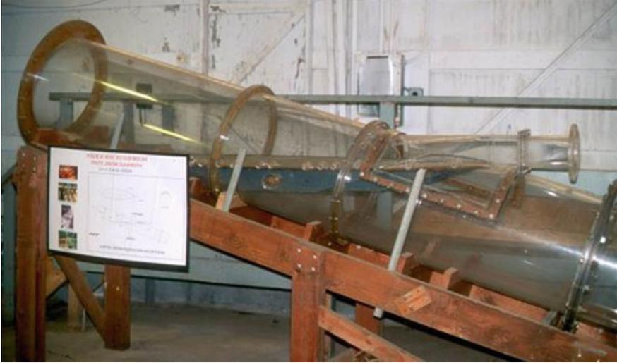
**Fig. 4.68** Eicher screen testing station at the hydraulic engineering facility of the Alden Research Laboratory in Holden (USA) (U. Schwevers)
