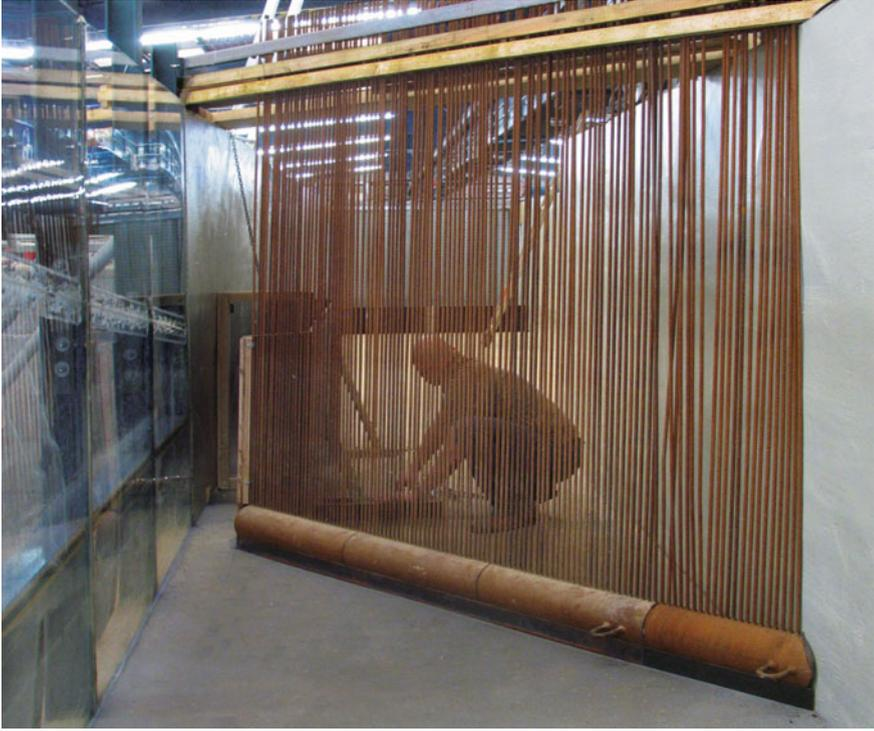
**Fig. 4.23** Installation of a chain bar at an angle of  $40^\circ$  in an ethohydraulic model flume, with a bypass on the left (B. Adam)
