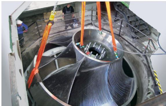
**Fig. 6.5** Runner of the Pentair Fairbanks Nijhuis turbine (adapted from Pentair Cooperation)
