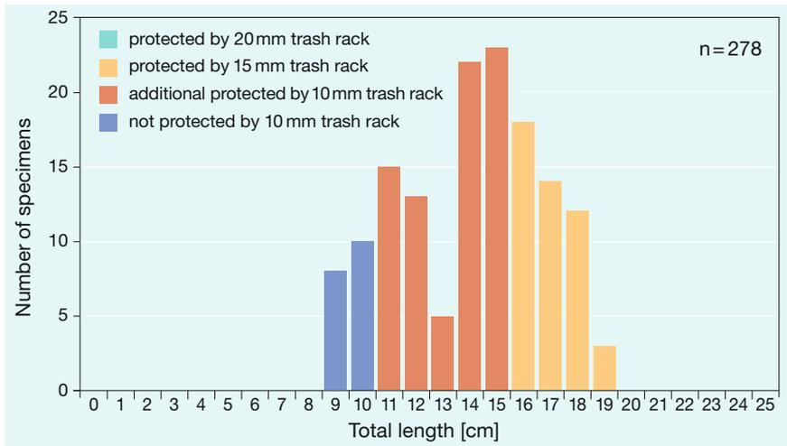
**Fig. 4.46** Frequency of lengths of migrating salmon smolts recorded by means of schokker catches in the Weser near Drakenburg in the 2009 season indicating the size classes which would be prevented from passing through bar screens of different clear widths (Schwevers et al. 2011a)
