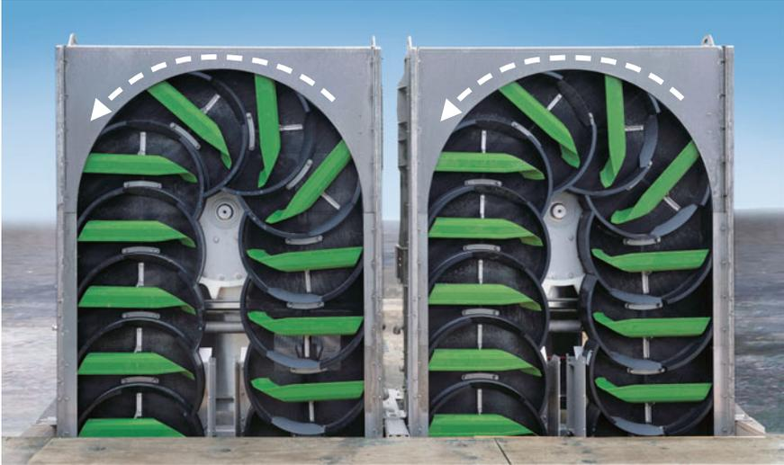
**Fig. 4.29** Apex of a MultiDisc™ screen. The black sickle-shaped mesh panels have green buckets attached which are supposed to carry fish to the return pipe; arrows mark the rotational direction (U. Schwevers)
