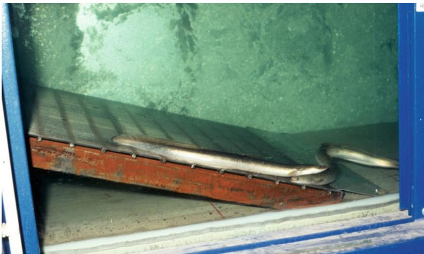
**Fig. 4.63** Ethohydraulic tests on eels on an inclined wedge wire screen. With  $v_a = 1$  m/s, the flow force vector acting perpendicularly to the plane of the screen is considerably reduced in comparison to a vertical screen, effectively preventing impingement (B. Adam)
