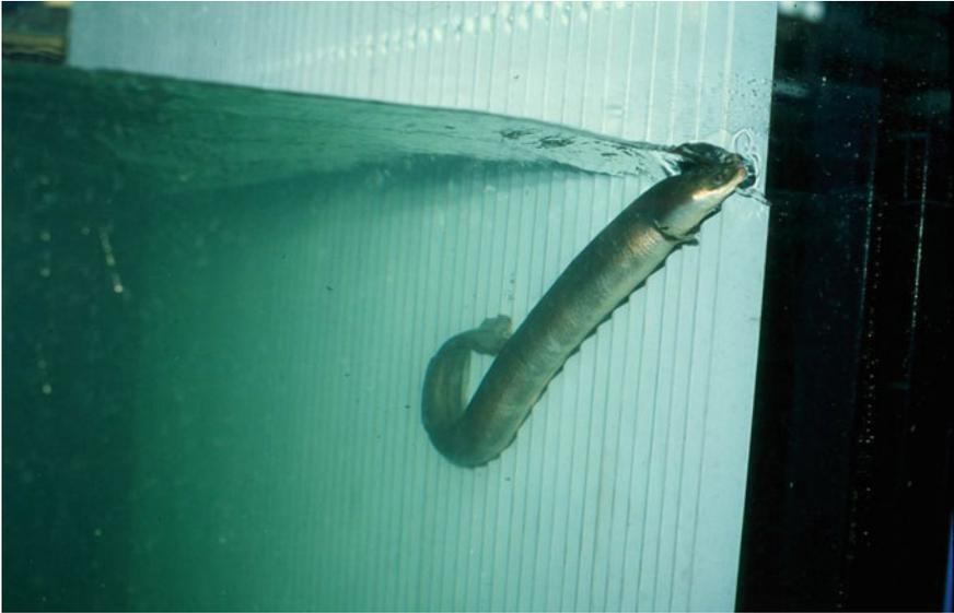
**Fig. 4.55** Eel impinging on a 20 mm screen in an ethohydraulic test with  $v_a > 0.5$  m/s (B. Adam)
