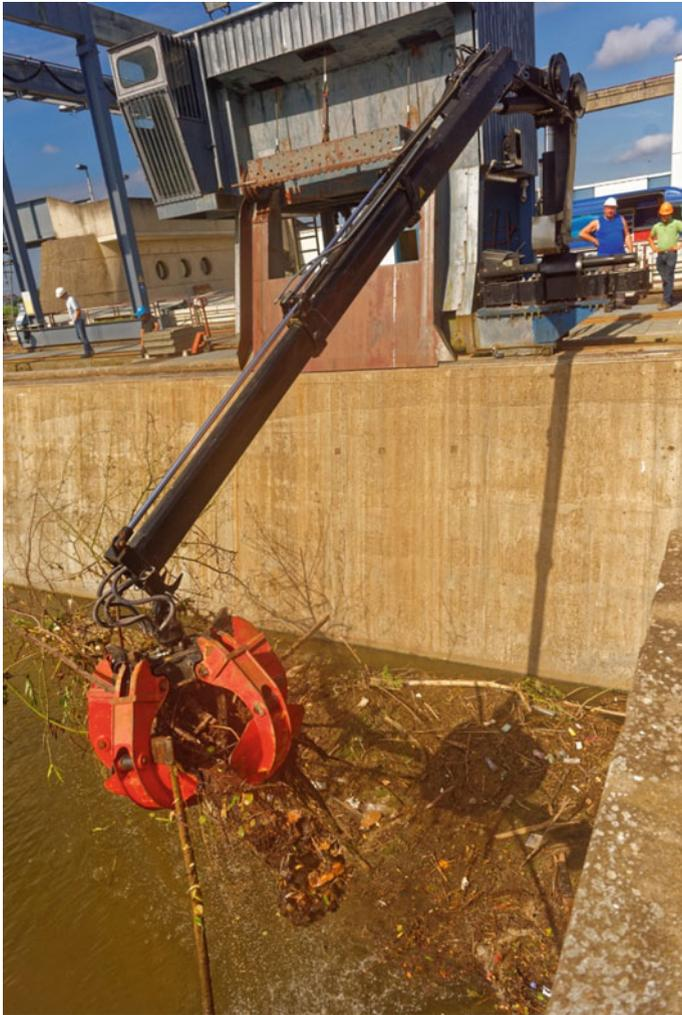
**Fig. 4.42** Hydraulic loading crane with orange peel grab for removing coarse debris (U. Schwevers)
