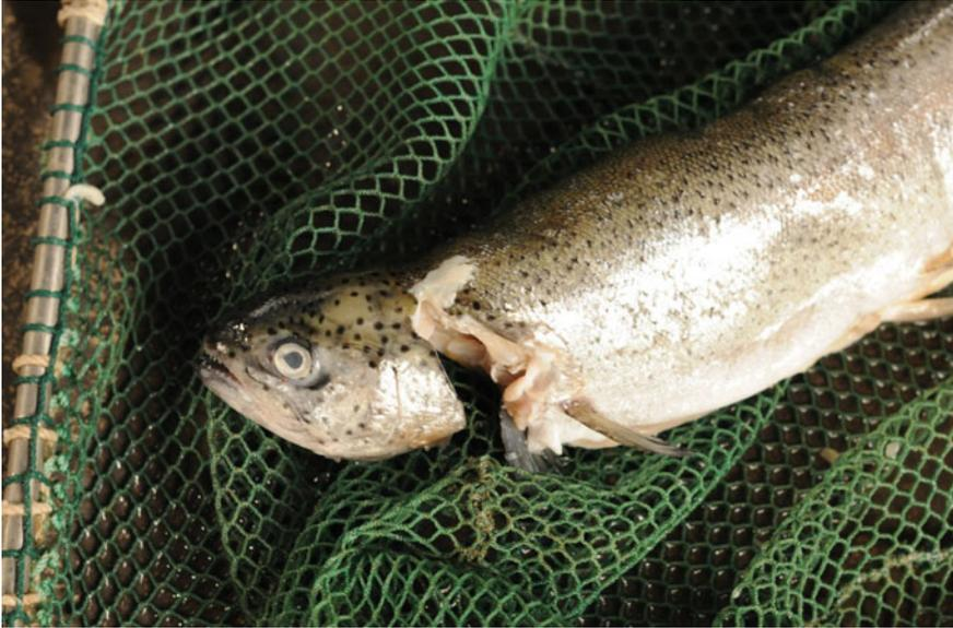
**Fig. 3.21** Partially severed head of a fish resulting from the descent of a water wheel's blade into its apron; dead rainbow trout were used as dummies in this ethohydraulic tests (B. Adam)
