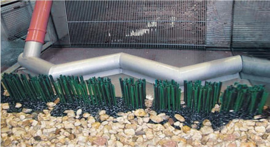
**Fig. 5.16** Zigzag pipe in combination with bristle bundles installed in a model flume transversely to the screen ([www.klawa-gmbh.de](http://www.klawa-gmbh.de); accessed October 01, 2015)
