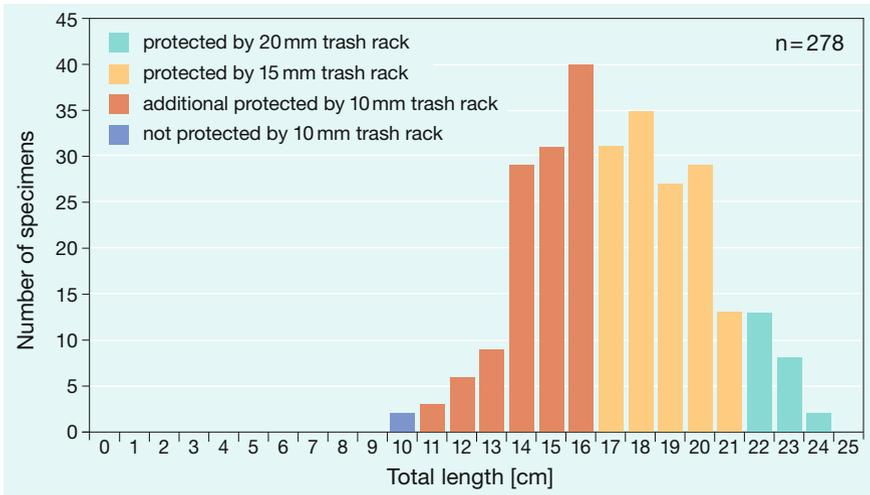
**Fig. 4.47** Frequency of lengths of migrating sea trout smolts recorded by means of schokker catches in the Weser near Drakenburg in the 2009 season indicating the size classes which would be prevented from passing through bar screens of different clear widths (Schwevers et al. 2011a)
